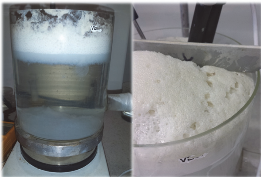
Fig. 11. EC-treated DWW (on the left) and resulting DWW sludge.
