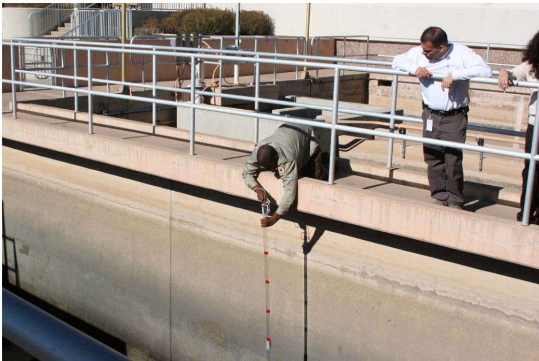
Filter assessment of filter media loss.
