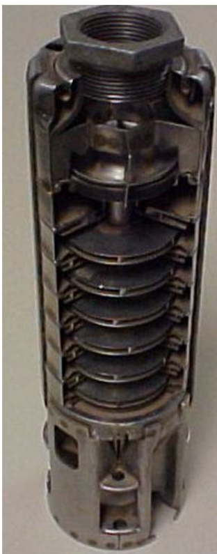
Cut away of a small submersible pump.
