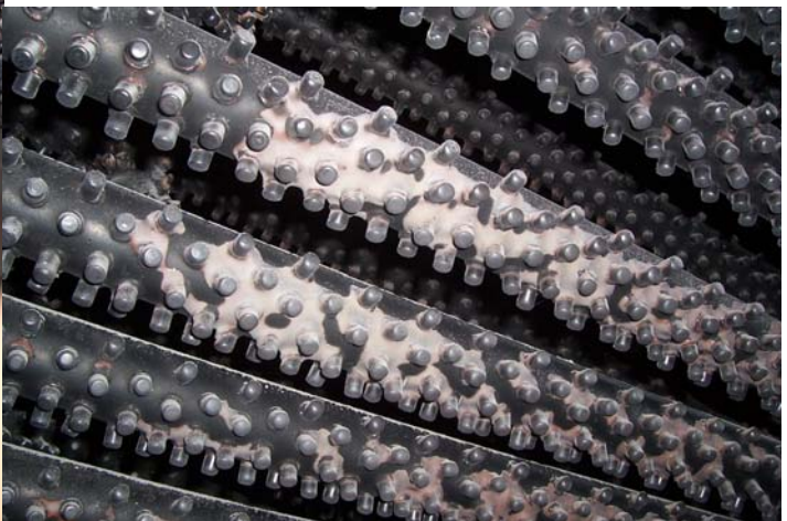
Photo 1-3: Photos above illustrate the ash fouling above coal nozzles. Blunting of outer studs is seen.
