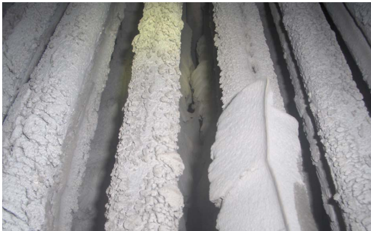
Case study 4- photo 1: deposition in a boiler fired with empty fruit bunches of palm fruits. This fuel contains more sodium and no chlorine. The superheater & economiser are coated with ash but corrosion failure was not reported.
