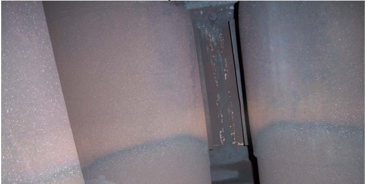
Photo 6: The whitish deposit seen at the weldment. The sparkling particles are seen above the normal water level. The dark colored water indicates that there had been high pH in the boiler water corroding the boiler.
