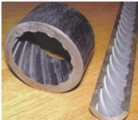
Photo 3- shows the internally ribbed tube / also known as rifle bore tube.
