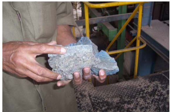
Photo 16: Ash molten in furnace due in adequate furnace size & waterwall surface.
