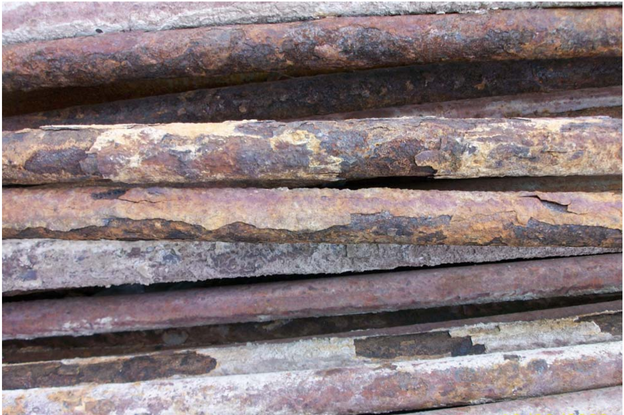
Case study 2: Photo-5: The corroded final SH coils removed from the boiler. The corrosion occurs due to action of KCl, NaCl at the high temperature zone where chlorine is able to deplete Cr as well as Fe.
