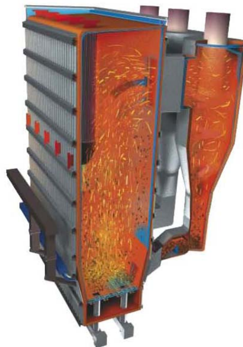
Figure 2: CFBC illustration with cyclone & loop seal.
