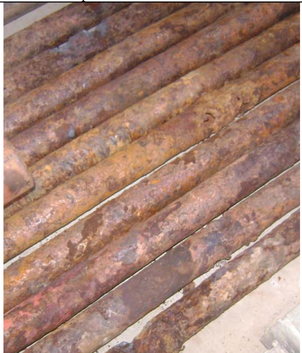
Case study 4: Photo -4: All Super Heater tube length removed from boiler showing the corrosion of the tubes. The first leakage had occurred near soot blower area.
