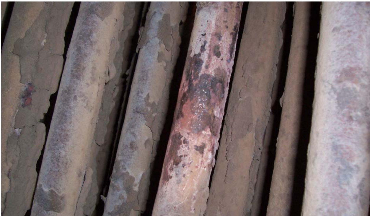
Case study 1: Photo 2- Ash deposition over secondary Superheater. Tube showing corrosion when the ash is removed.
