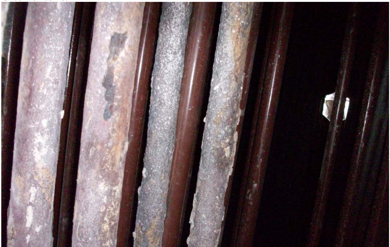
Case study 2: Photo - 6: Corroded final superheater coils along with new coils at the rear.
