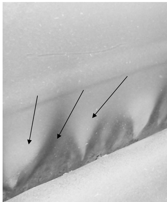
Photo 2: Marks of outside air ingress below water drum in a boiler
