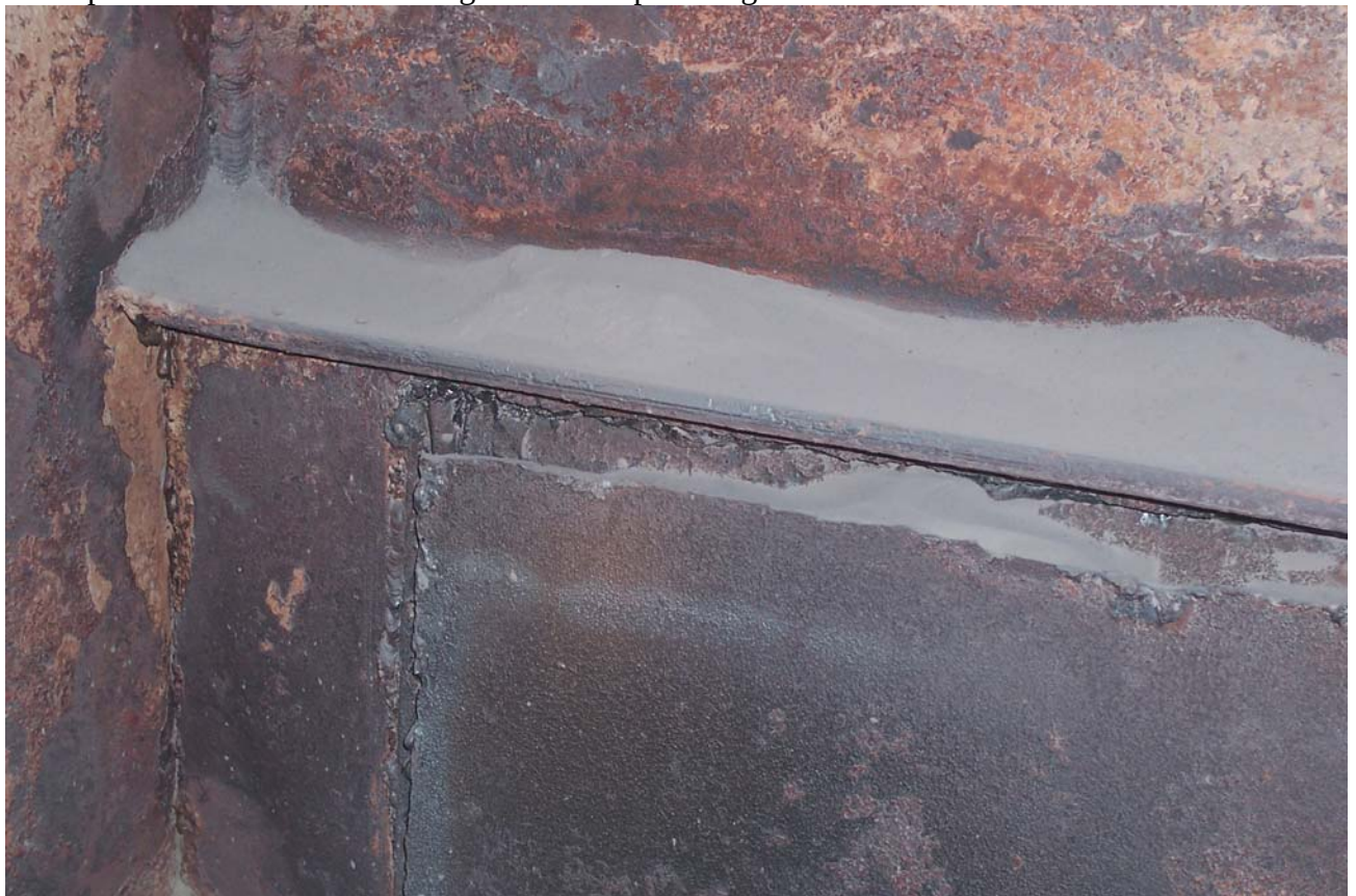
Photo 17: The top row of economizer tubes are provided with impingement shields. The second row is not provided with such an arrangement. The polishing of tubes are seen in the second row.
