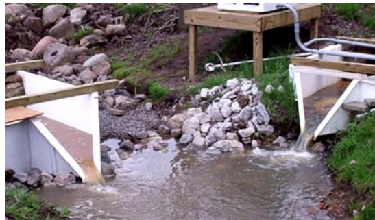
Figure 2.15 – Typical H-Flume Application 14
