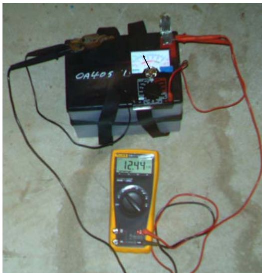
Figure 4.1 – Digital and Analog Meters on a Partially Discharged Battery (12.44 volt reading)
