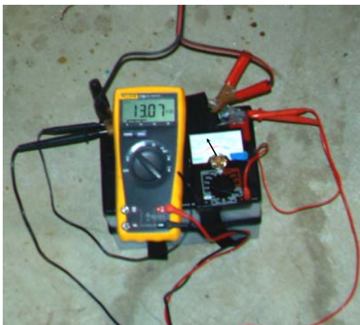
Figure 4.2 – Digital and Analog Meters on a Battery Being Charged (13.07 volt reading)
