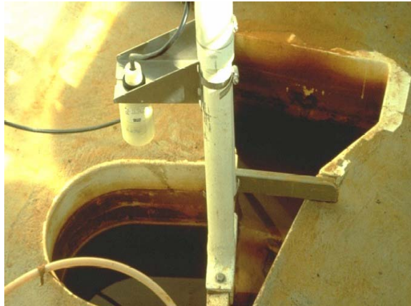
Figure 2.16 – Ultrasonic Sensor, Mounting Bracket, and Stilling Well 15
