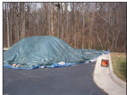
Figure 11. Salt pile covered with a tarp.
