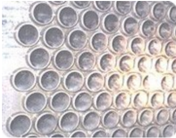
Tube after 300 hours operation with ATCS
