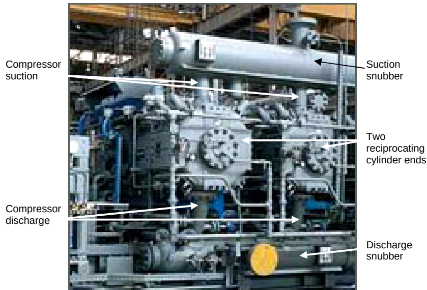
Figure 4.5: Suction and Discharge Snubbers—Two Cylinders in Parallel
