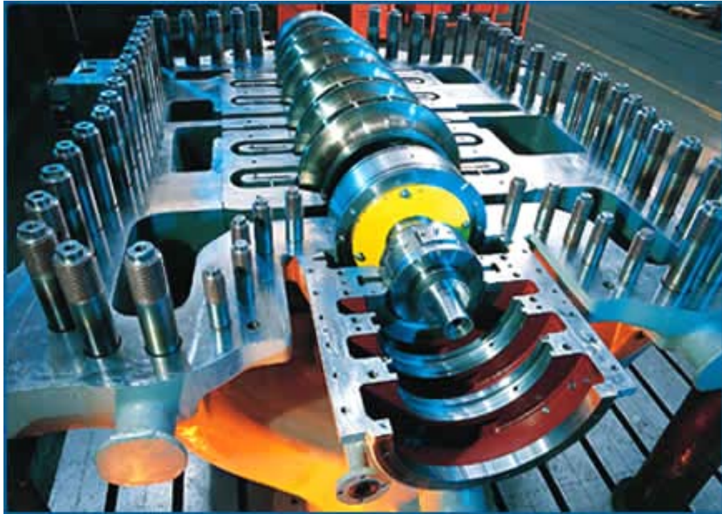
Figure 5.12: Horizontally-split Compressor with Upper Casing Removed
