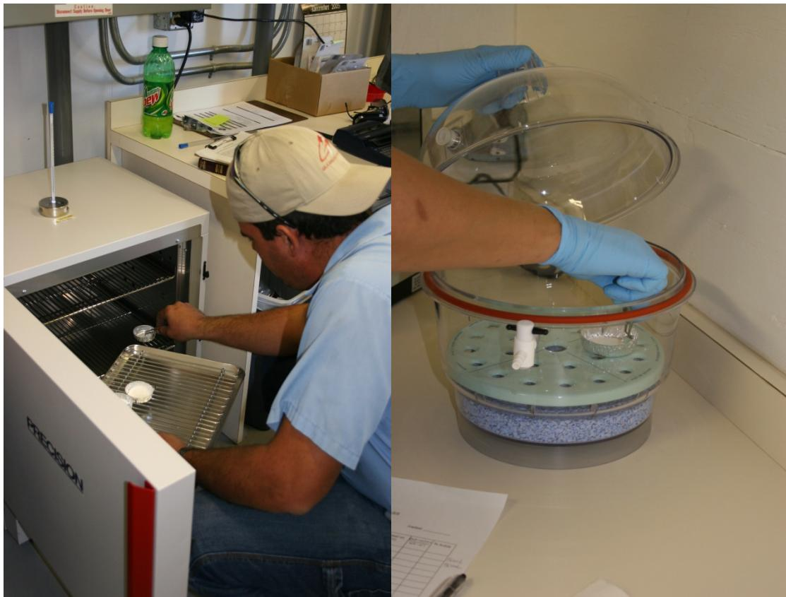
Top left, filters being baked at 105°C. Right photograph, filters in desiccant.
