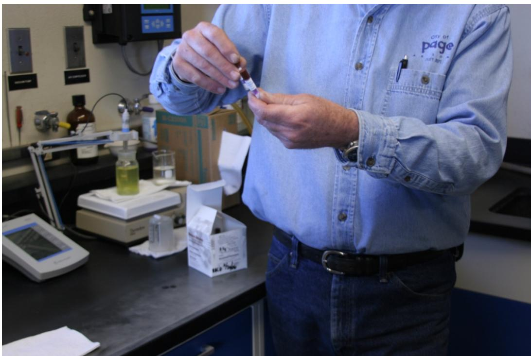
The tubes held in this photograph should be placed in an autoclave. One tube is a standard or QA and the other would indicate contamination.
