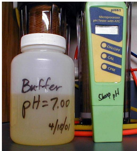
pH Meter pH scale is between 0-14 0 being Acid and 14 being Base. For fun, we measured Orange Juice and that is pH 3.5 or so - acid! We also measured Welch's Grape Juice and the meter showed 3.4 - also an acid (and slightly stronger). Here is a close-up of the pH41 meter we use and its pH 7.0 buffer solution (used for calibration and storage - there are a few drops of the buffer solution in the cap of the pH41 to keep it properly moist when not in use).
