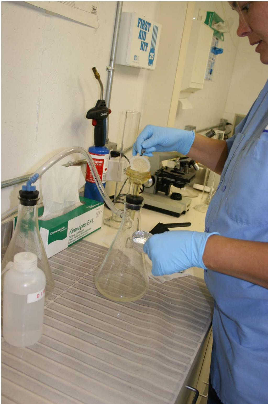
Lab tech removing filter for TSS analysis.
