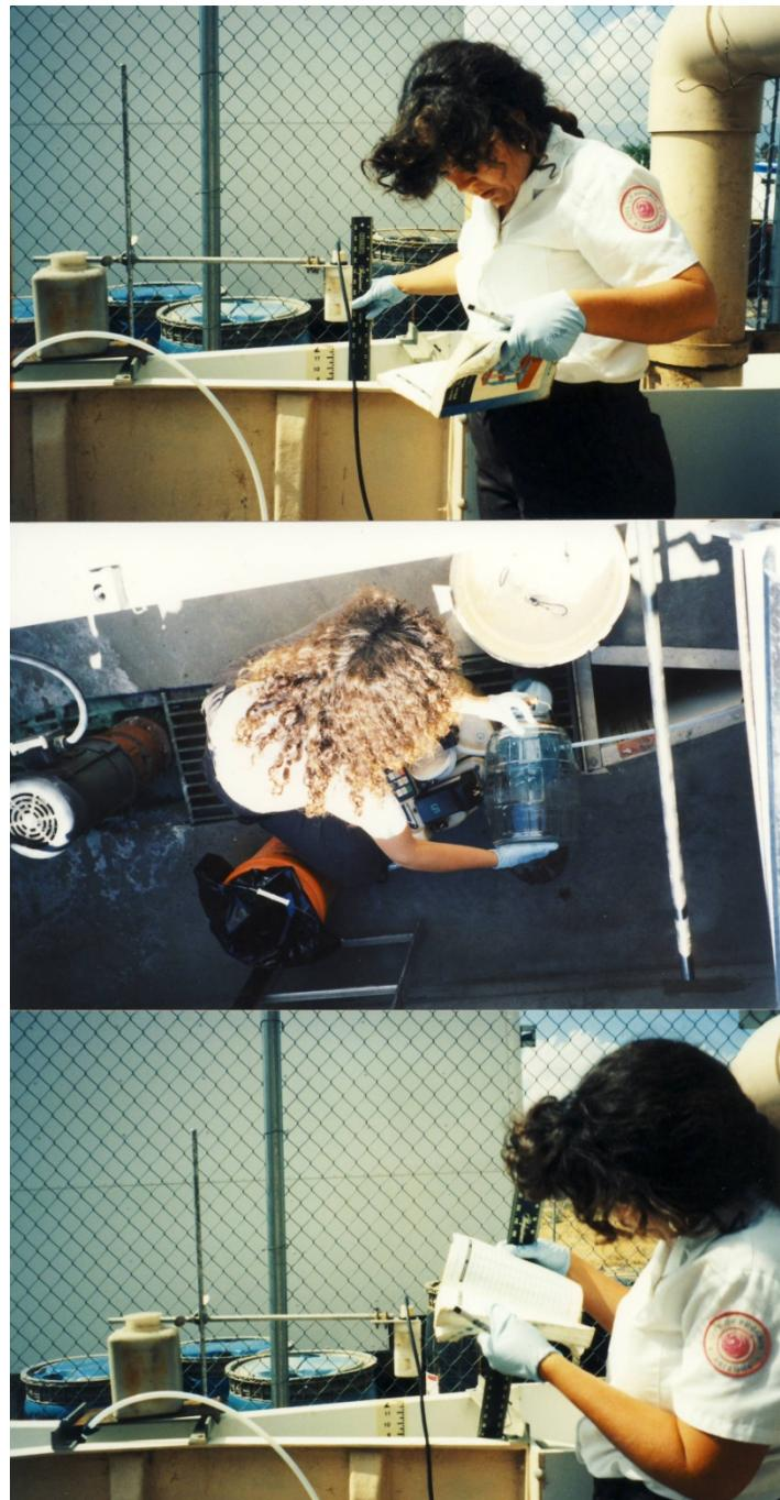
Here is a wastewater Inspector is utilizing the auto sampler's manual to help adjust the time and adjust for the correct flow for a composite sample. You can see that she is pouring off the pickle jar. This inspector is also the course author.
