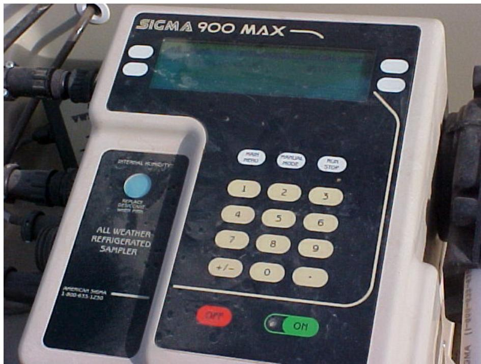
The refrigerated automatic WWT sampler will have a Data programmer that will allow you to set the time to collect the sample or samples. This machine can also measure the amount of the sample. These can also be used for the collection of composite samples. Sometimes you will see a pH probe with real-time readings sent to the Operator's Command Center. These are a common sight at most wastewater plants and SIUs.
