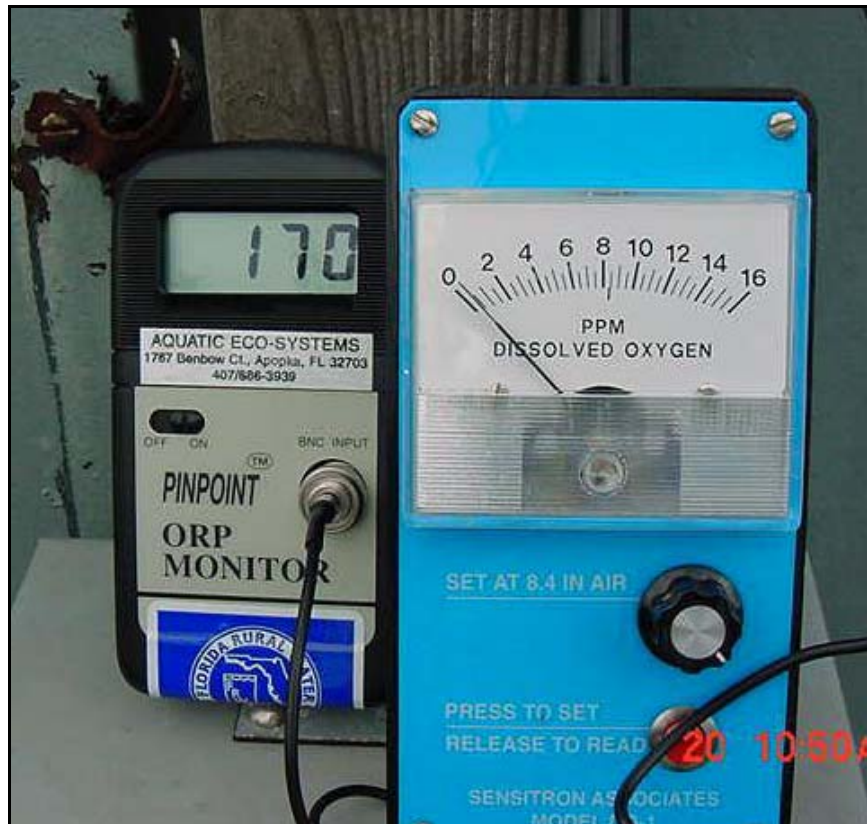
Figure 16: ORP meter (on left) and DO meter
