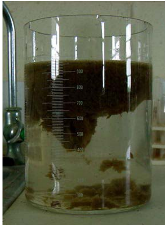
Figure 13: Settleometer with mixed liquor that has risen, or ‘popped-up’
