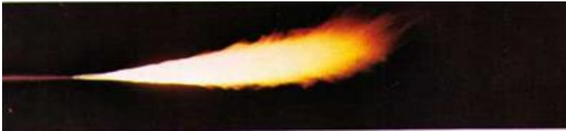
Acetylene burning in air Not suitable for welding.
