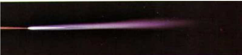
Strongly Carburizing Flame Metal boils and is not clear.
