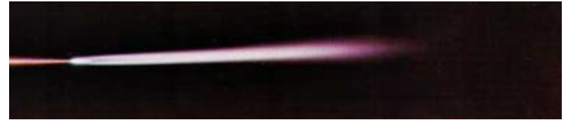
Slight Excess Acetylene Flame Similar to neutral flame – little or no puddling is necessary.
