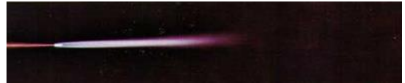
Neutral Flame Metal is clean and clear, flowing easily.
