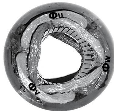
Figure 2: Distributed winding inside stator
