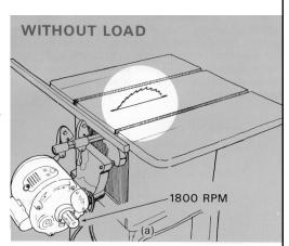
Synchronous Speed =  $\frac{120 \text{ x Frequency}}{\text{# of Poles}}$
