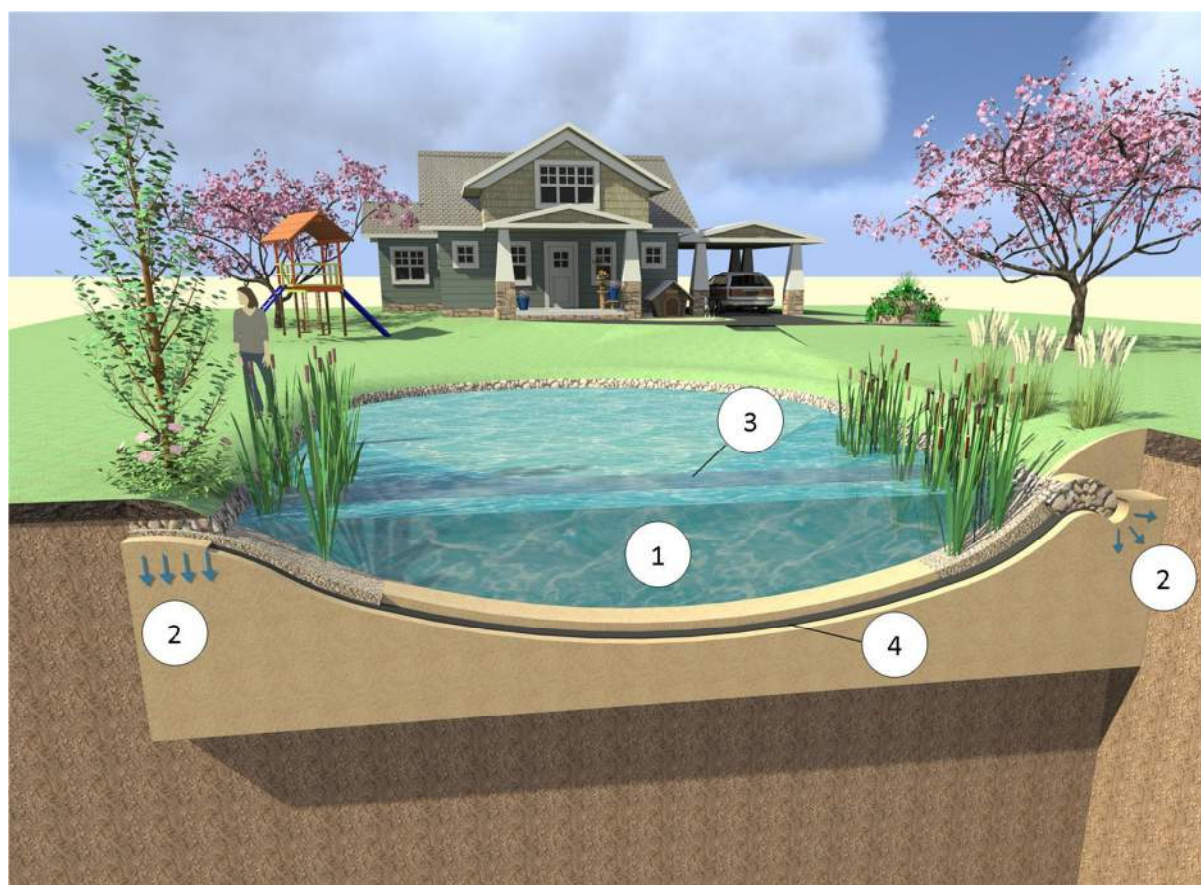
Figure 4.7 Small Water Reservoir with Retention Space and Bank Infiltration. ( Retention space = area where it is possible to move water level )
