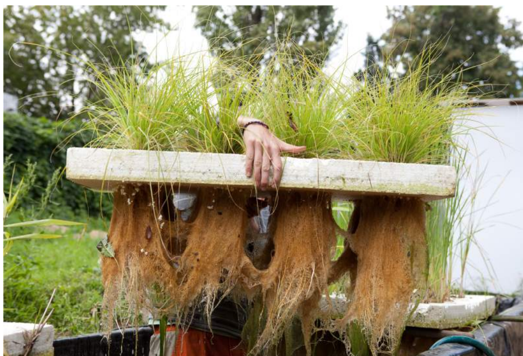
Photo 16: Artificial floating wetland with extensive root system developed after six months of operation
