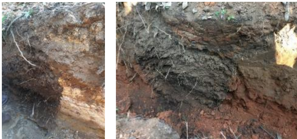
Figure 6-10: Photos demonstrating clustering of roots in and around buried sludge, likely due to elevated nutrient levels
