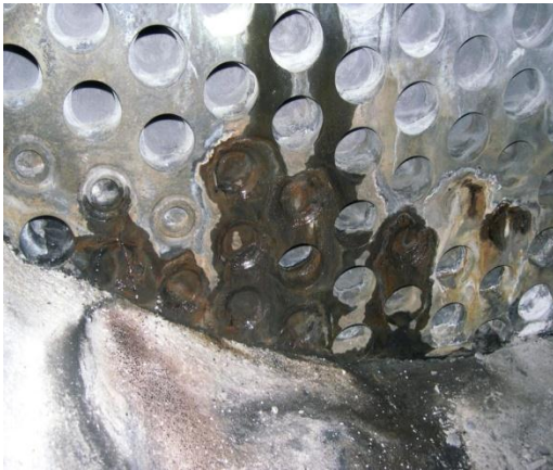
Figure 9 and 10: Cracks in outlet tube sheet
