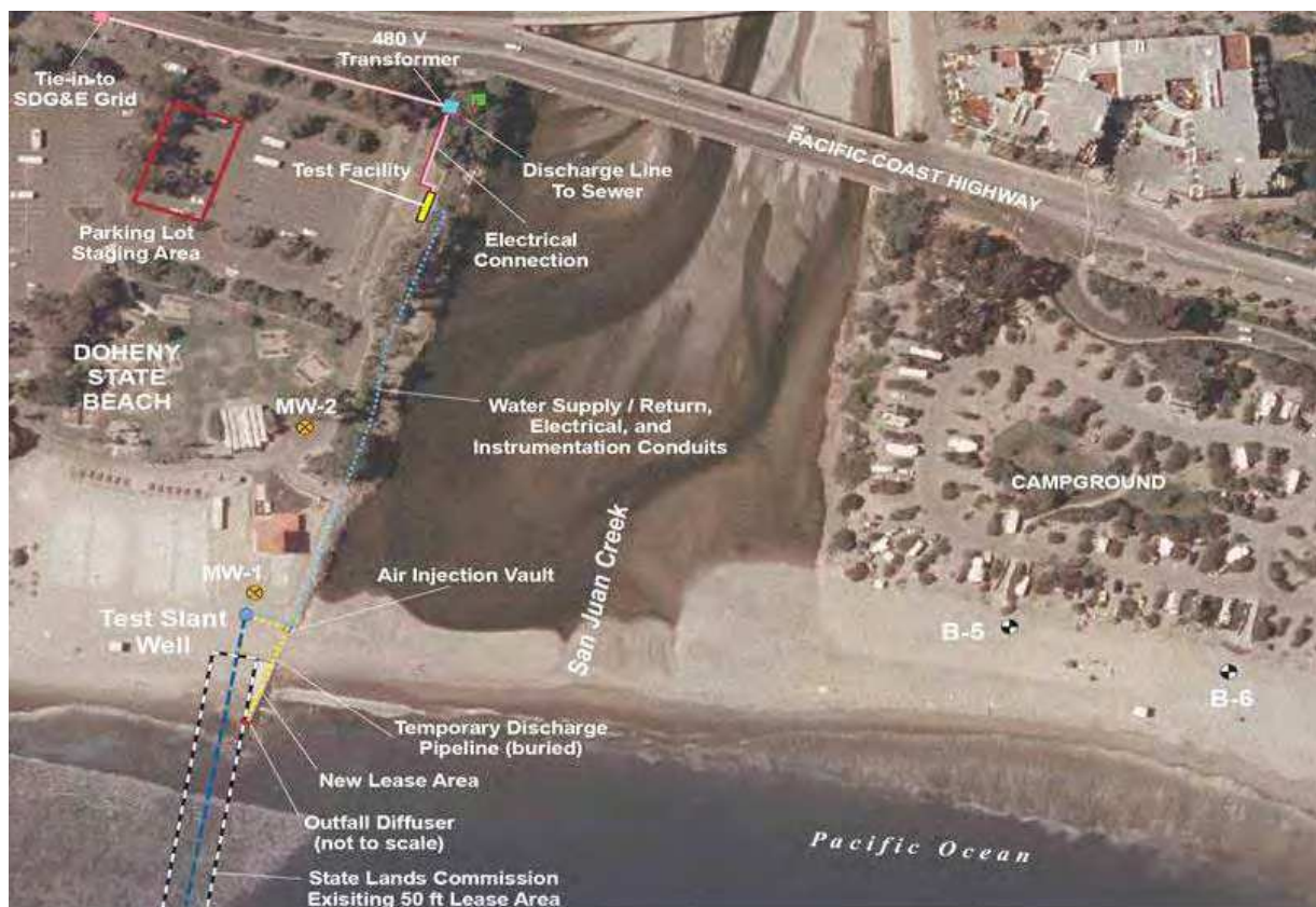
Figure 9.3 Phase 3 extended pumping and pilot plant testing facilities, Doheny State Beach, feasibility investigation, Dana Point Ocean Desalination Project
