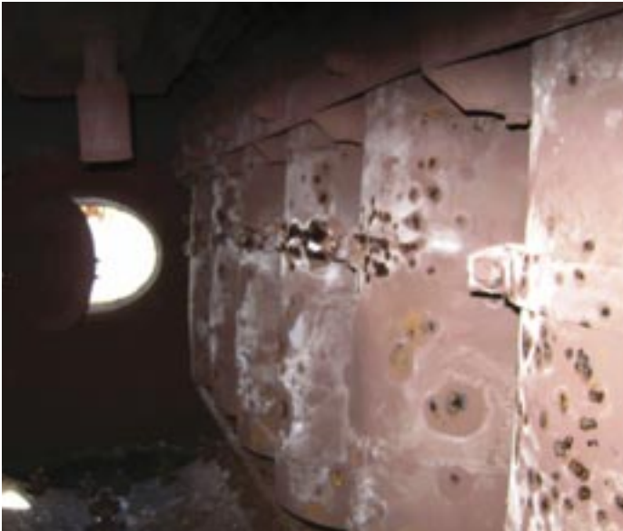
Pitting corrosion on steam drum separators, likely caused by a deficient wet layup. Cortec® image.
