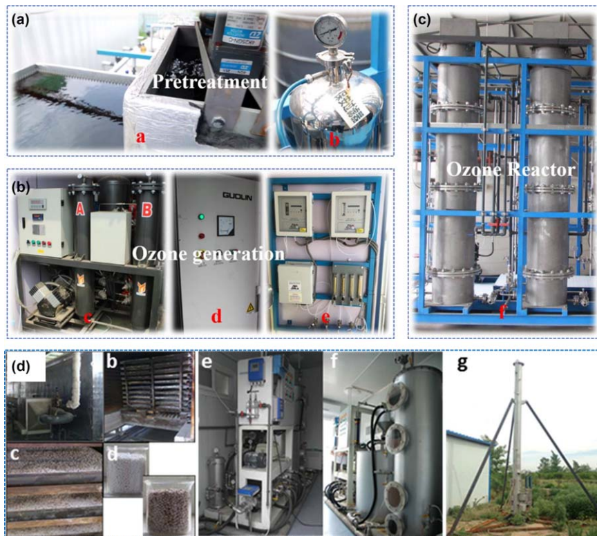
Figure 2.8 Pilot-scale units for catalytic ozonation: (a) coagulation sedimentation and cartridge filtration, (b) oxygen generator, ozone generator, and ozone detector and gas flowmeters, and (c) a pair of cylinder column reactors for ozone reactions (the left one filled with CuCo/NiCAF, the right one empty for blank control). Reproduced from ref. 91 with permission from American Chemical Society, Copyright 2019. (d) Photographs of the large-scale production of Mn-CeO x /γ-Al 2 O 3 catalysts and two-stage ozone oxidation towers for the pilot-scale catalytic ozonation of real wastewater. Reproduced from ref. 81 with permission from American Chemical Society, Copyright 2018.
