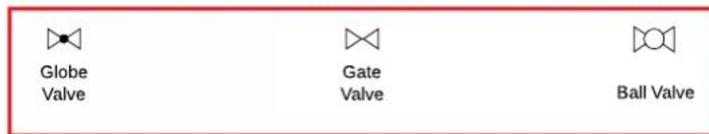
Figure 6.2 - Showing 3 Manual Valves, namely Globe, Gate, and Ball Valves
