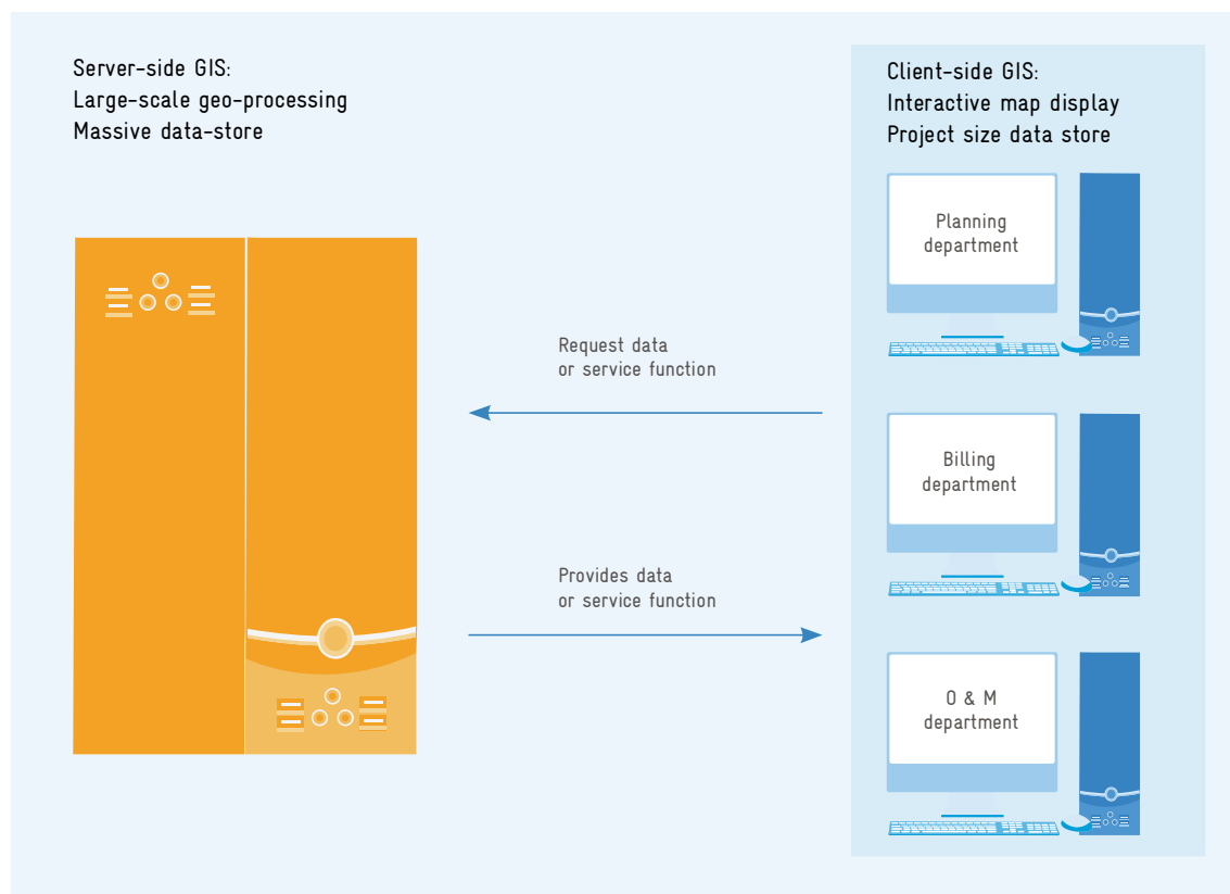
Figure 5.2 Client-server architecture for an enterprise-level GIS, based on [93]
