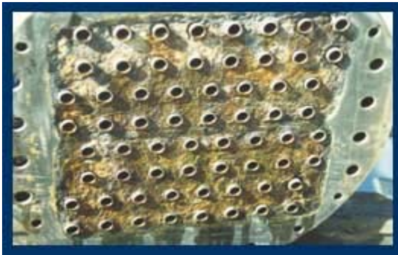
Scaled Heat Exchanger Tubes
