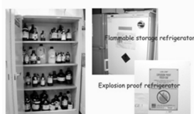
Store flammable chemicals in flammable storage cabinet or explosion-proof/flammable storage refrigerator
