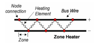
The output ratings of these cables depend on the resistance of nickel alloy wire and the amount used between node connections. Consequently, manufacturers standardize the output wattages to specified values. These cables can be cut to any convenient length in field within the limits imposed by the maximum heating circuit length (typically 160 to 320 ft) and minimum bus-bar connection interval. When terminated the last 2-foot heater
