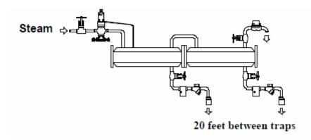
Distance between Traps (Jacket Pipe); Fig. Source: Spirax Sarco
