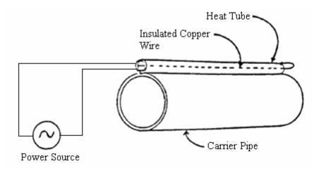
When the system is powered by high voltage (3 to 5kV), heat output occurs in both conductors. If the system is properly designed, 60 to 80% of heat output takes place in the steel tube, and only 20 to 40% in the inner conductor.
