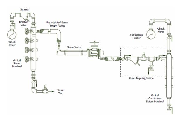
**Typical Steam Tracing System (Figure Source: Thermon)**
