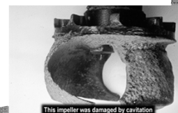
This impeller was damaged by cavitation
