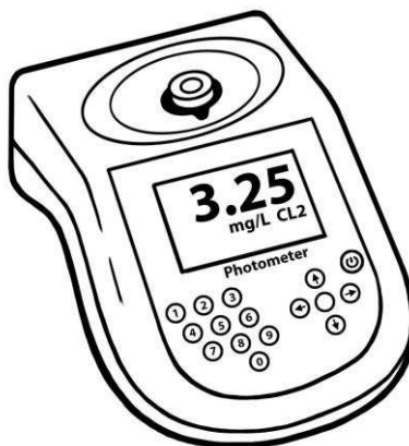
Photometer used to measure chemicals in water
