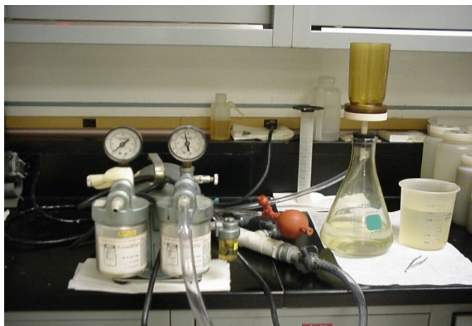
Lab equipment used for determining Total Dissolved Solids.
