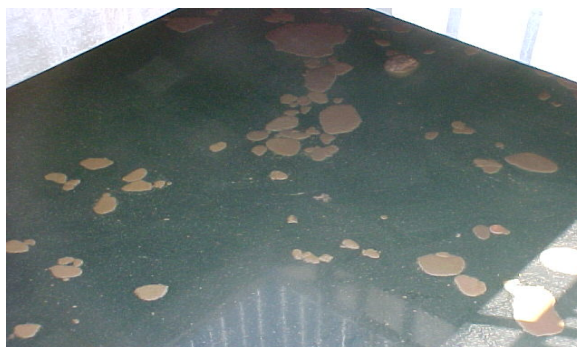
Floating clumps of floc in the flocculation compartment.
