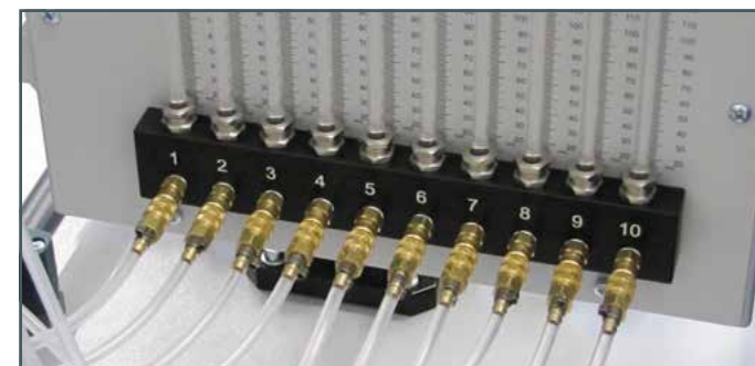
Connections on the manometer panel for measuring the pressure in the filter bed
