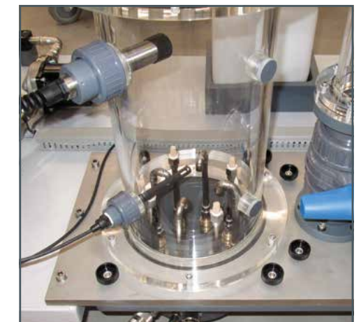
Various distributors for aerating the reactor
