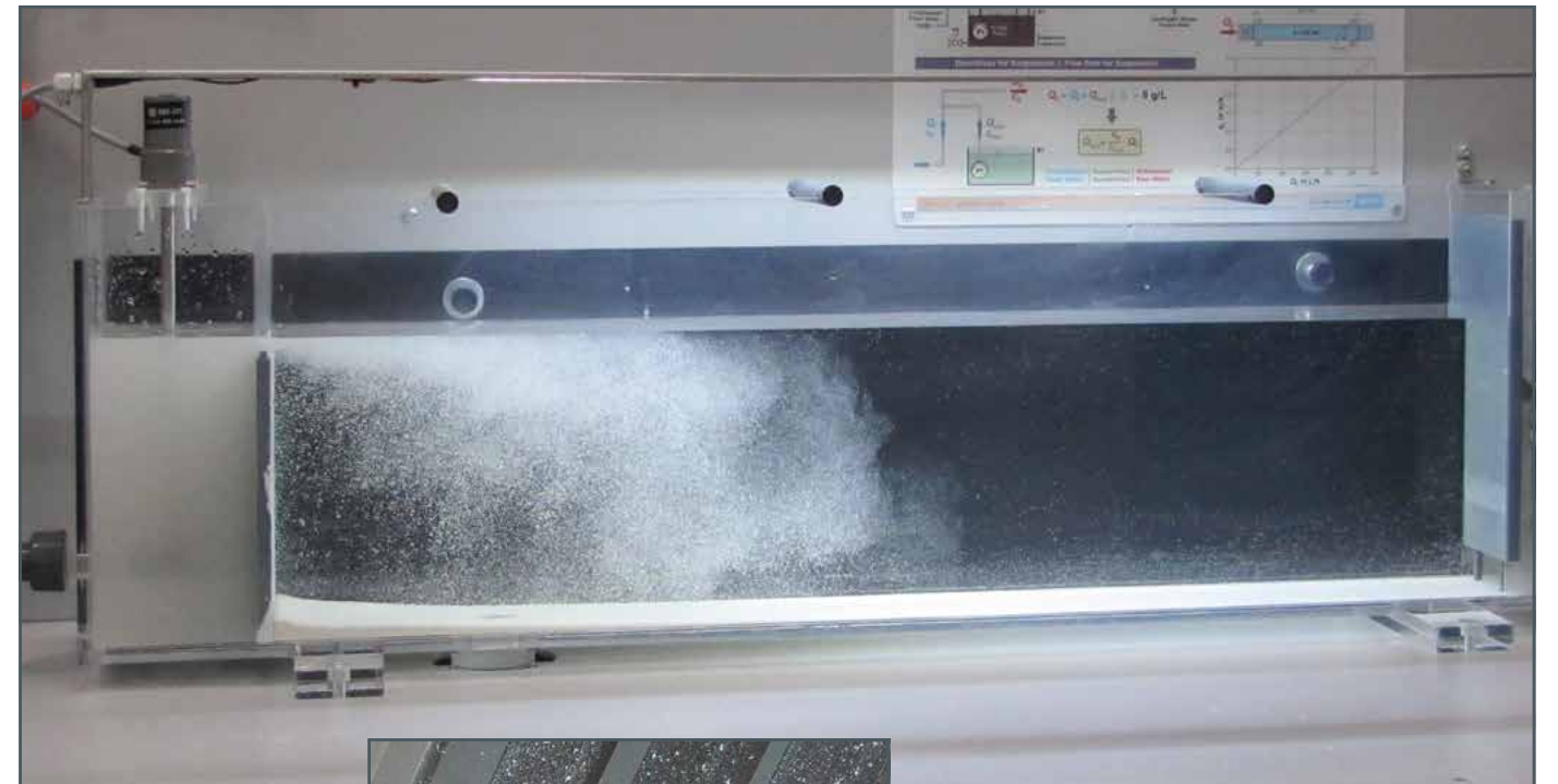
The sedimentation process and the flow conditions can be observed very clearly thanks to the use of transparent materials and lighting.
