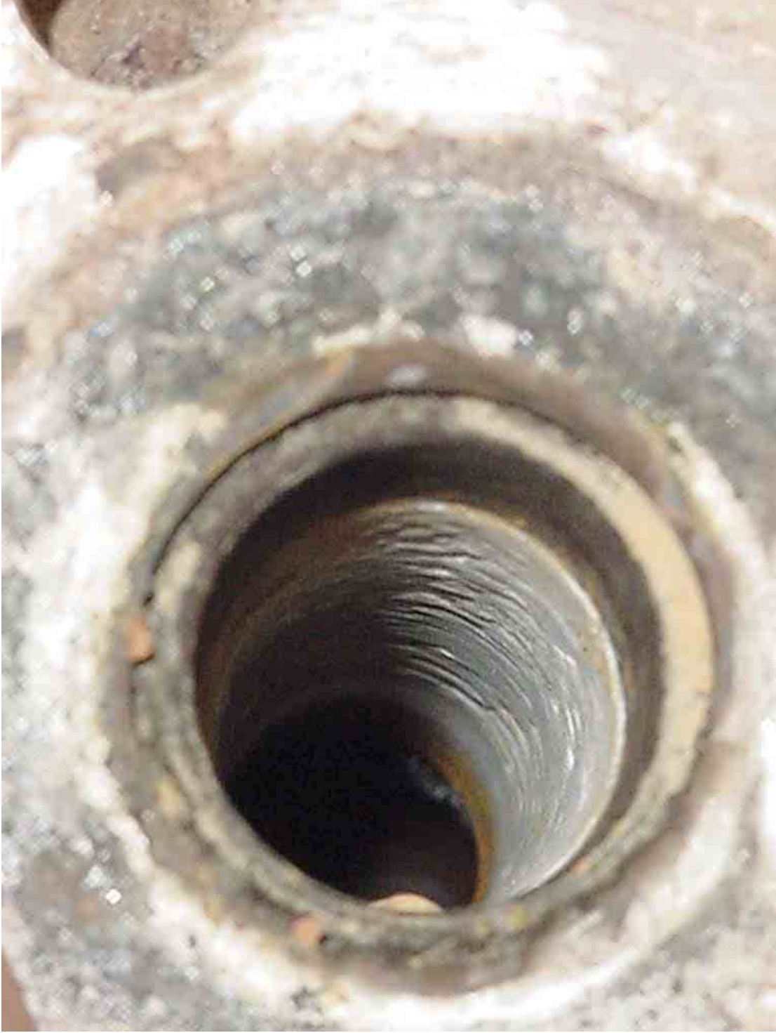
Figure 38 Fouled surface of high flux heater following repeat tests on Device A
