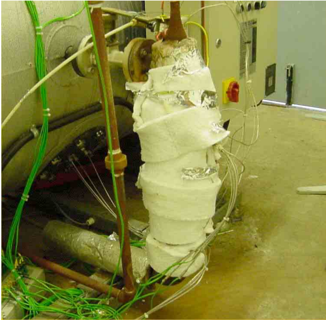
Figure 7 Electrically heated vertical tube section during application of insulation
