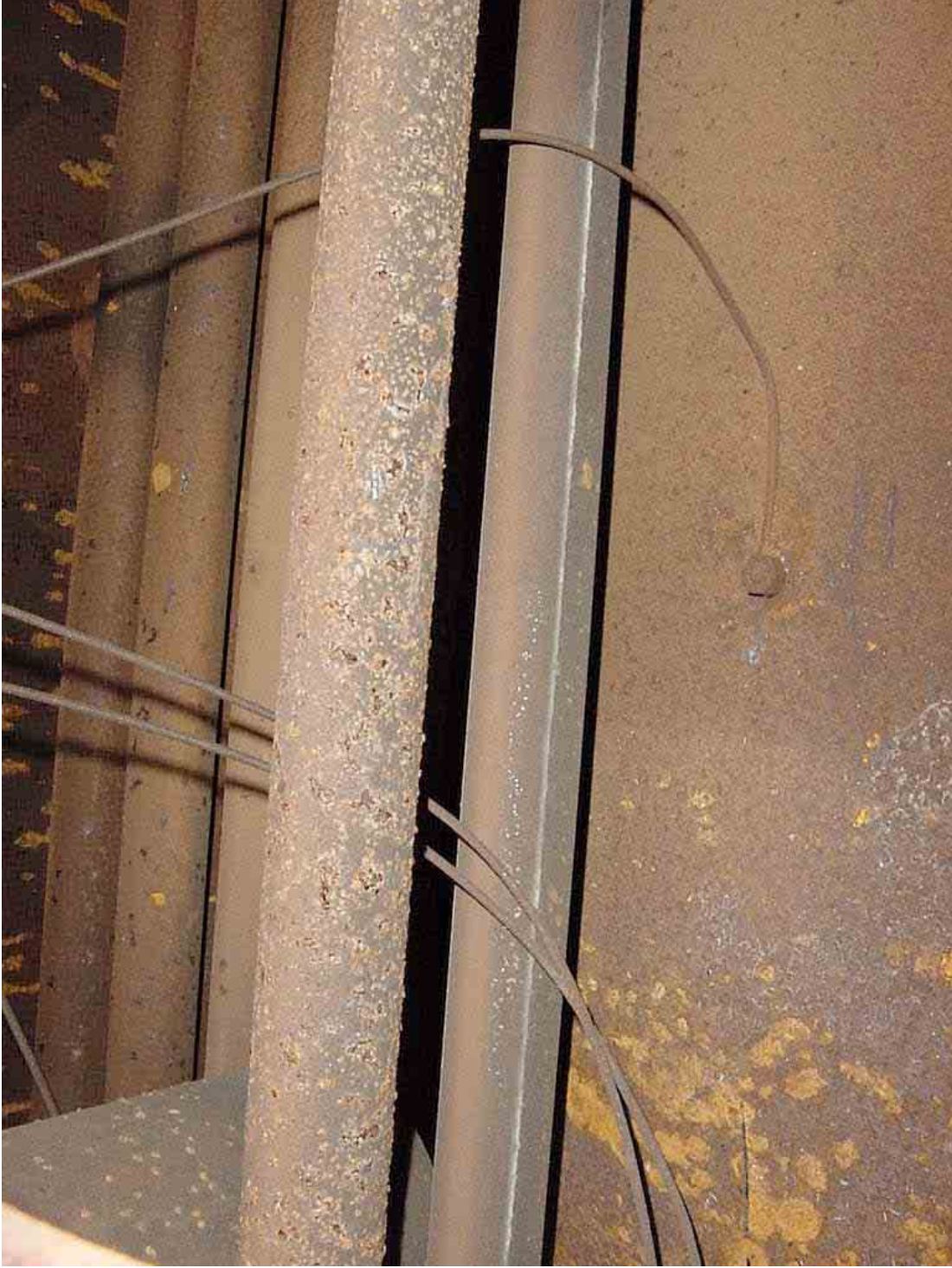
Figure 34 Boiler surfaces after repeat tests on Device A
