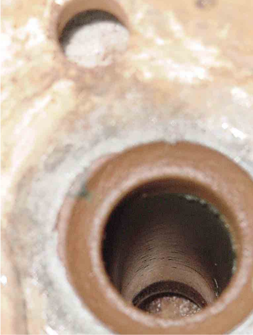
Figure 28 Interior of high flux heater after trials with Device D
