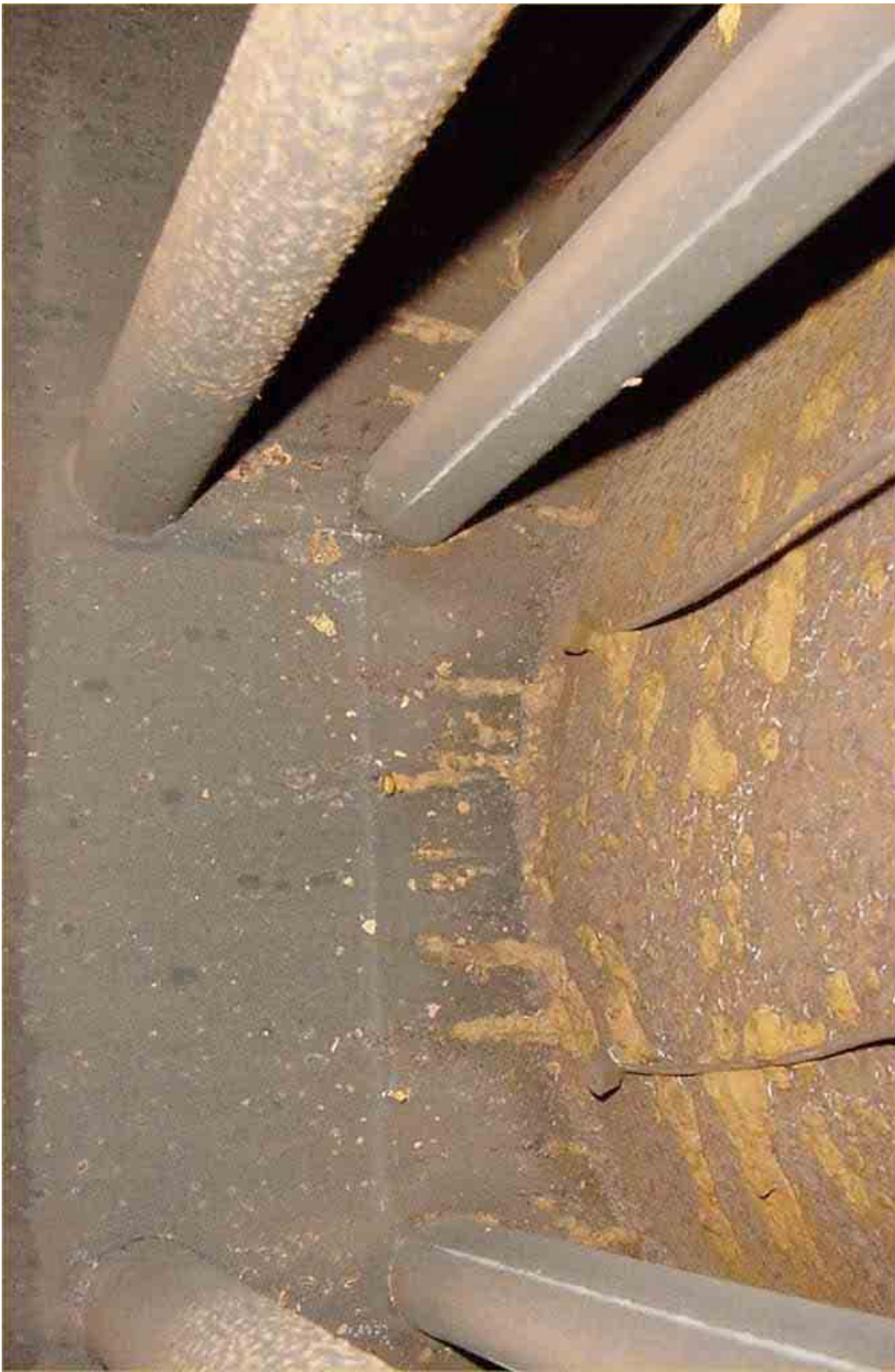
Figure 35 Boiler surfaces after repeat tests on Device A
