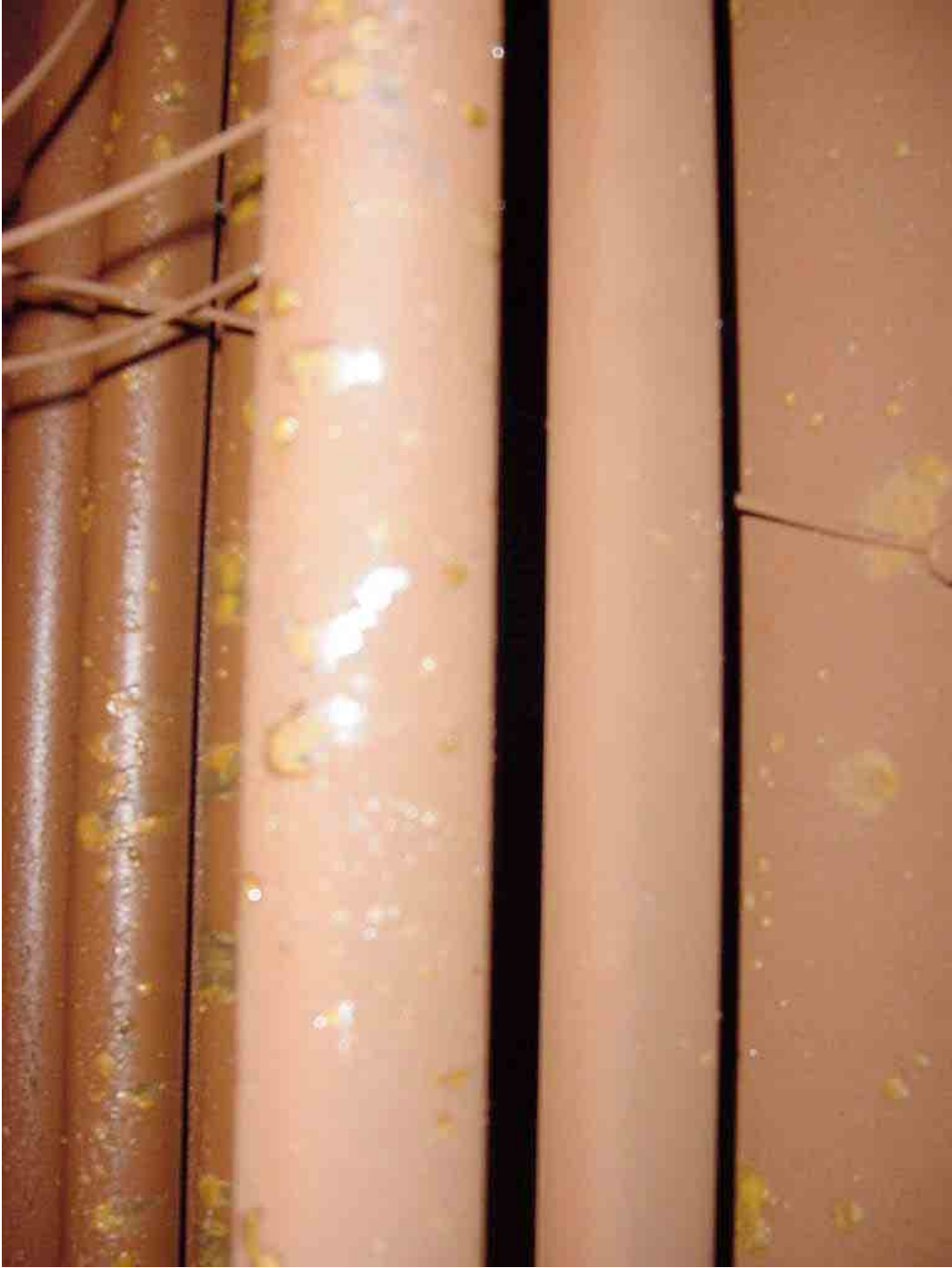
Figure 14 Smoke tubes after untreated runs
