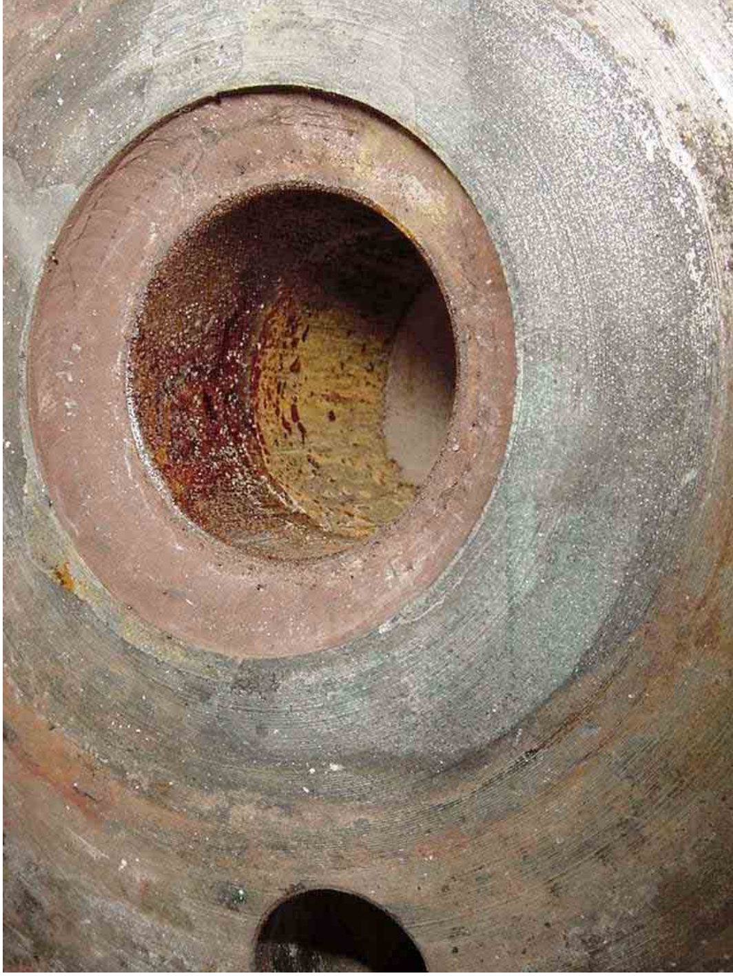
Figure 26 Interior of high flux heater after untreated runs
