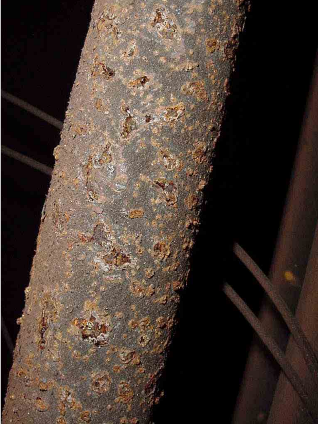
Figure 36 Close up of stay tube following repeat tests on Device A
