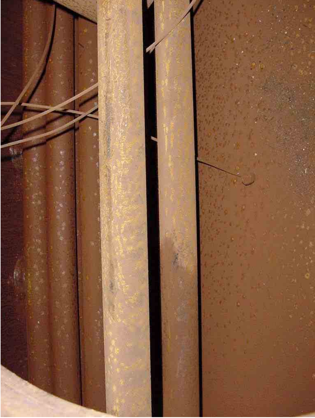
Figure 24 Smoke tubes after tests with Device D
