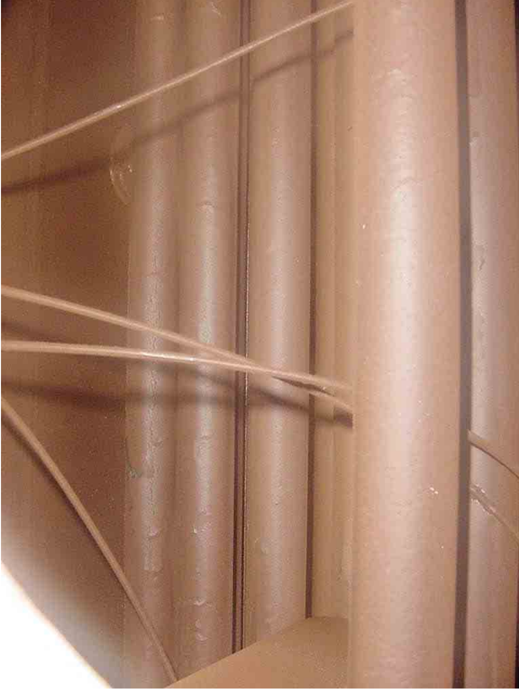
Figure 16 Smoke tubes after tests with Device A
