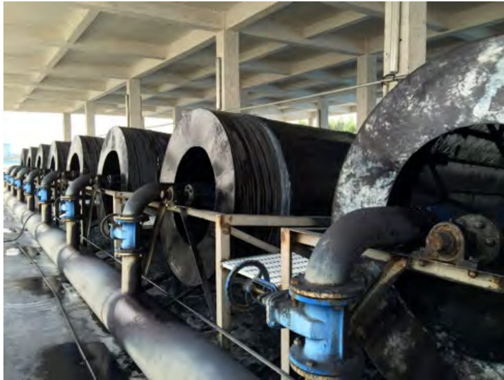
Figure 12: A row of drum screens in a textile effluent treatment plant
