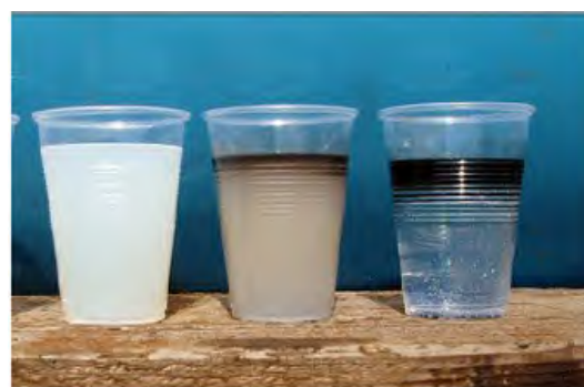
dissolved oil emulsified oil separated oil
