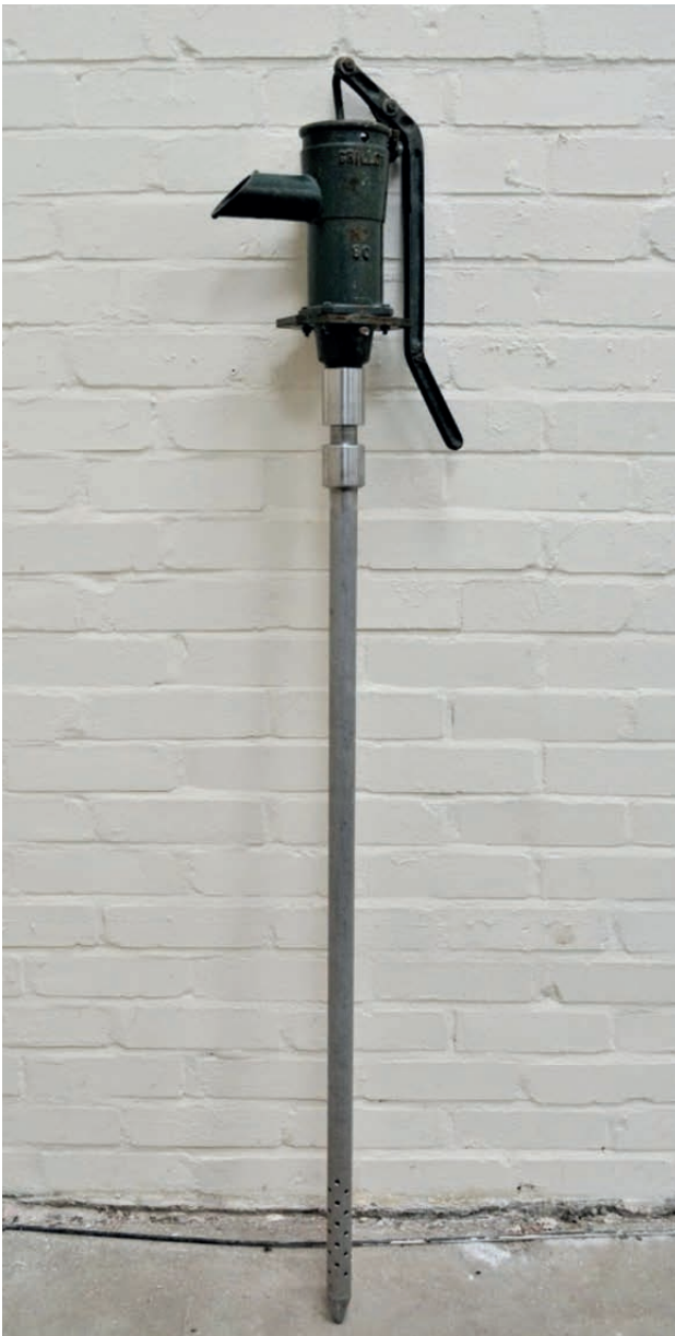
Figure 4.7 Bou-Rouch pump and standpipe
