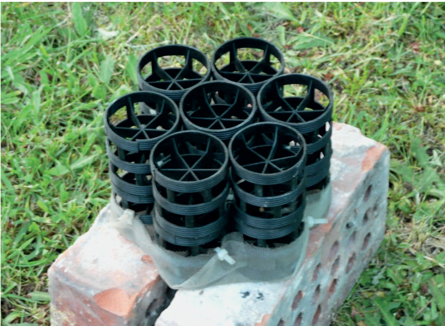
Figure 4.5 SAufU artificial substrate
