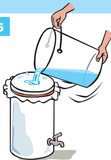
Pour the treated water into a container through a clean cloth filter.
