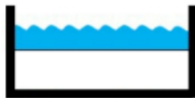
A. Rectangular weir without end contractions
