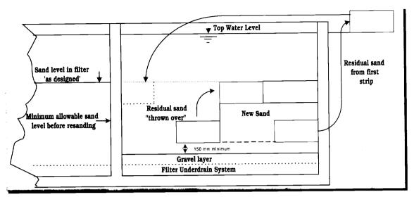
FIGURE 4: REASANDING A SLOW SAND FILTER USING THE TRENCHING METHOD
