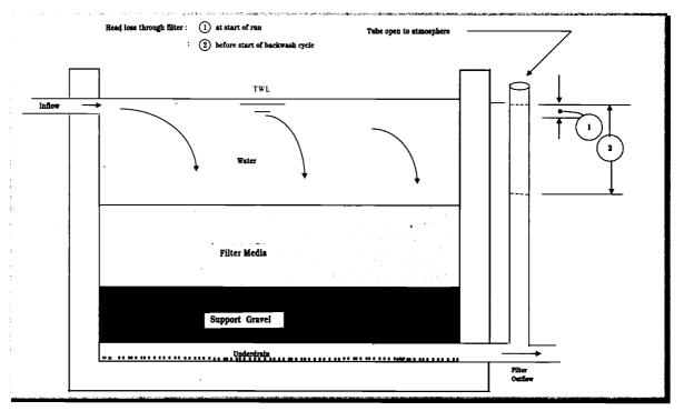
FIGURE 9: MEASUREMENT OF HEADLOSS
