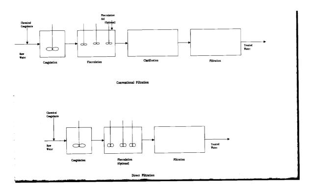
FIGURE 5: CONVENTIONAL AND DIRECT FILTRATION
