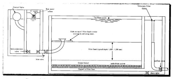
FIGURE 3: SLOW SAND FILTER AND PREFILTRATION CONTROL CHAMBER
