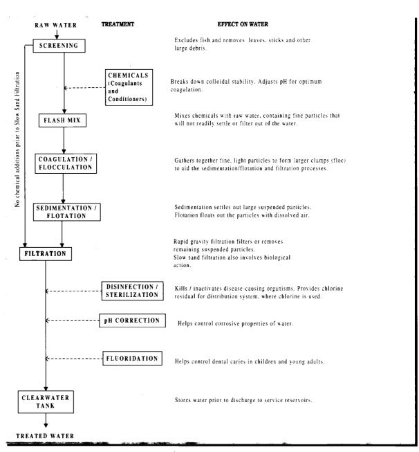
FIGURE 1: TYPICAL WATER TREATMENT PROCESSES
