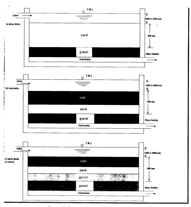
FIGURE 7: GRAVITY FILTER MEDIA CONFIGURATIONS
