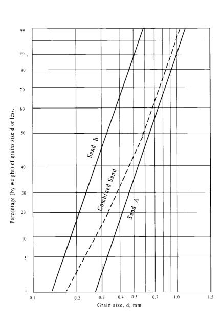
FIGURE 2: COMBINATION OF TWO TYPES OF STOCK SAND
