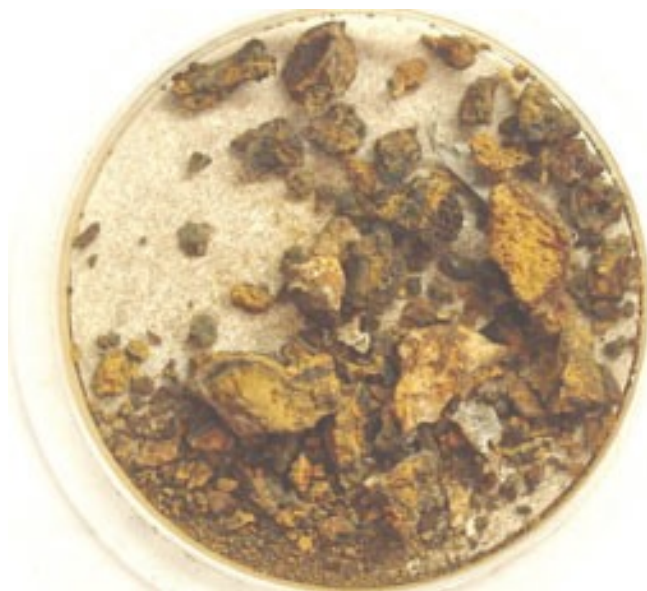
Large Rust Particles
