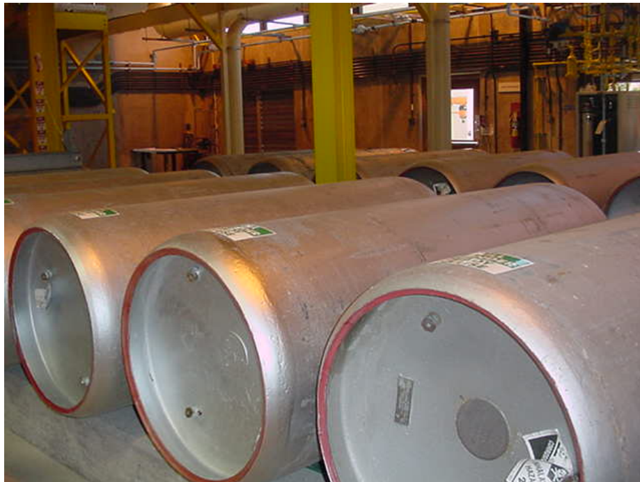
1-ton chlorine containers, rear side of container.
