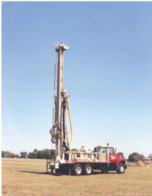
Typical Rotary Rig
