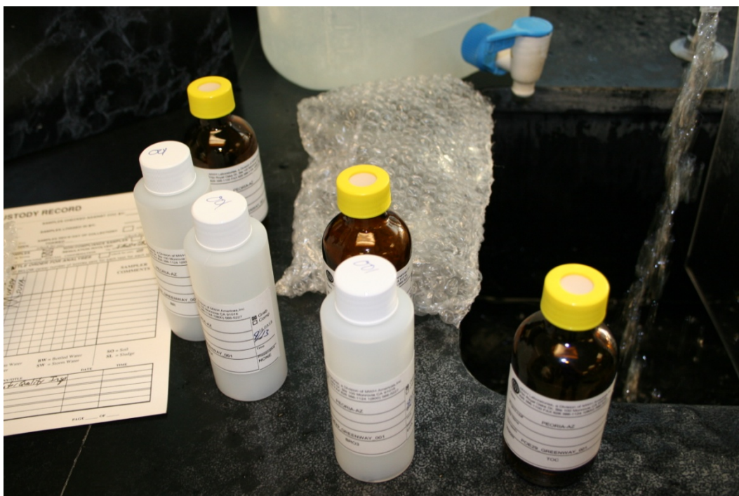
Various water sample bottles and chain-of-custody form.
