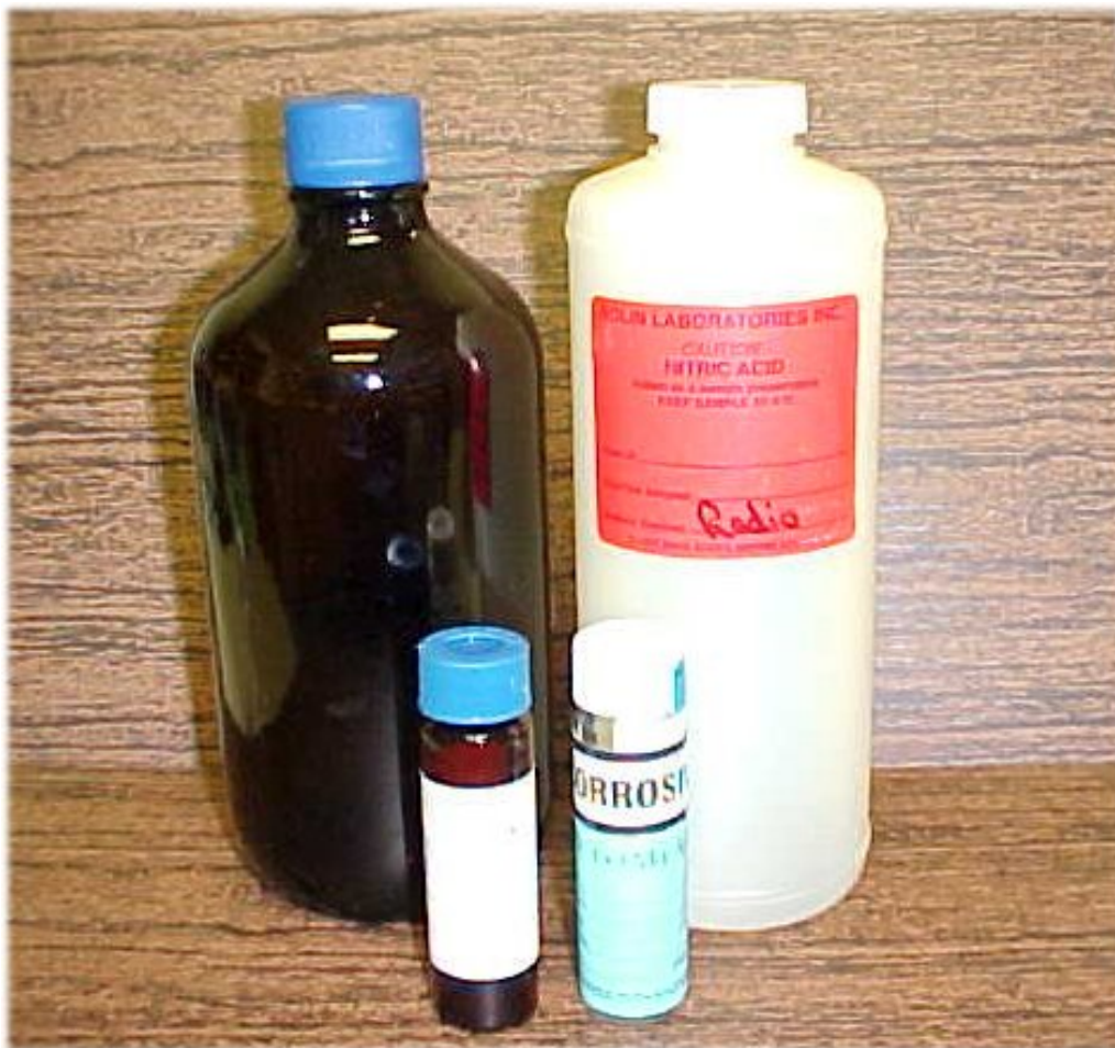
Common water sample bottles for distribution systems.
