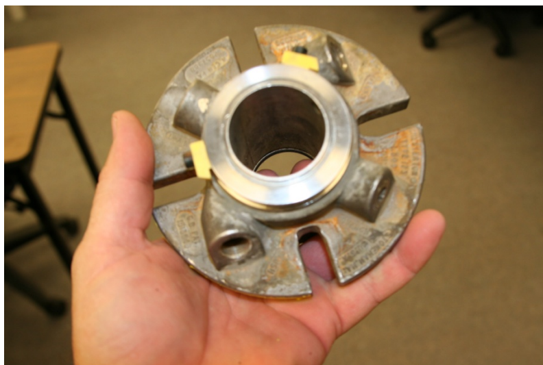
Vertical Turbine well with a mineral oil cooled seal. Mechanical seal bottom.
