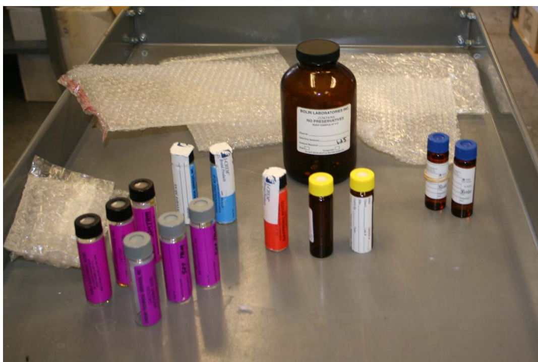
Various water sample bottles and chain-of-custody form.
