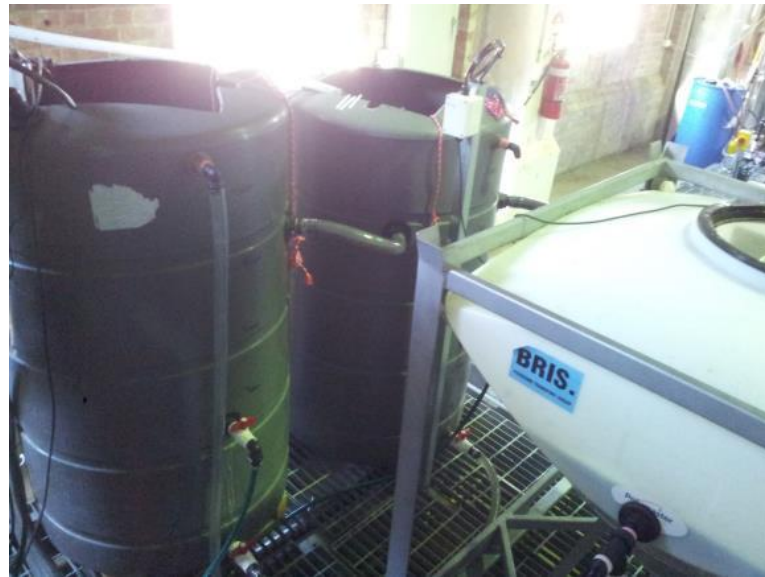
Figure 46. The two MBBR anammox tanks and clarifier for separating and returning suspended sludge.
