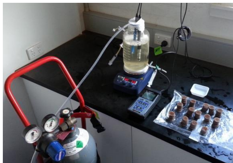
Figure 33. Preparation of a batch test for determination of anammox activity.
