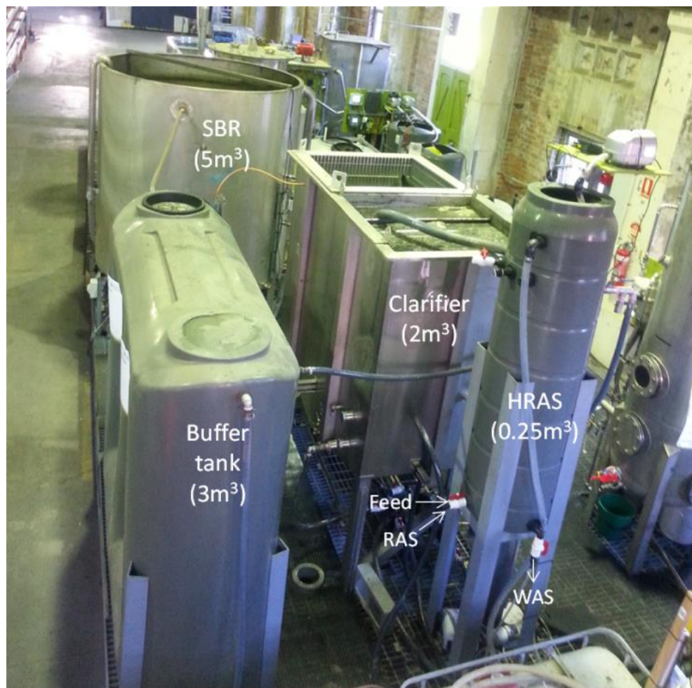
Figure 21. The first part of the aerobic treatment train: A stage (HRAS + lamella clarifier), and B stage (buffer tank + SBR).
