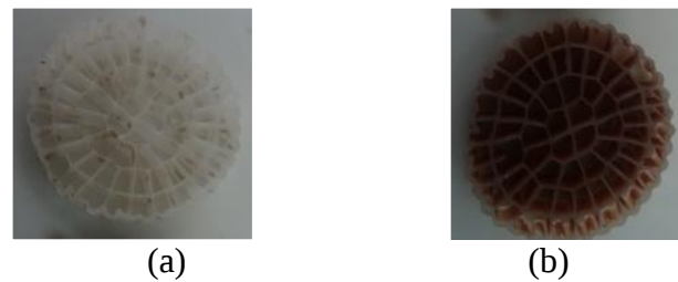
Figure 32. Anoxkaldnes K5 media; (a) new and (b) colonized with anammox bacteria grown on sidestream.
