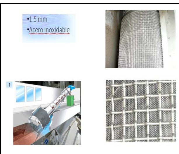
Figure 8. Mili-sieves for the pre-treatment
