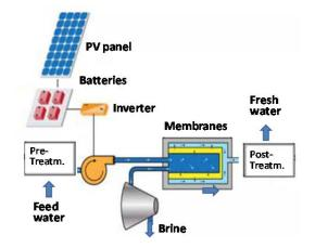
Figure 6 - Coupled PV and RO desalination plants (Al-Karaghouli et al., 2011)
