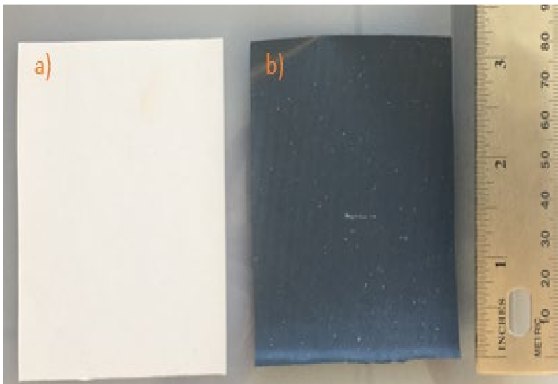
Figure 5. Membranes fabricated by custom phase inversion process: a) plain (Plain_0.0_Y_250), and b) doped (C-Cu_0.8_Y_250)
