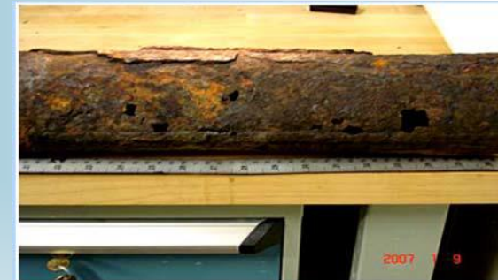
Corrosion damage seen on pipe
