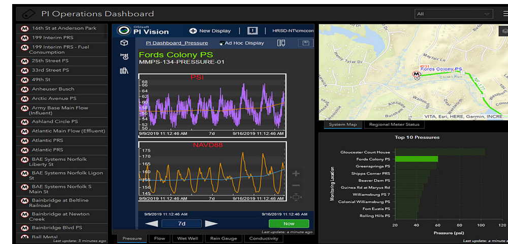
Hampton Roads Sanitation District visualizes real-time data from its OSIsoft PI data historian, Telog data logger fleet, and ArcGIS.
