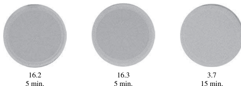
FIGURE 9.5 Iron accumulation on SDI test pads due to coagulant overdosing.
