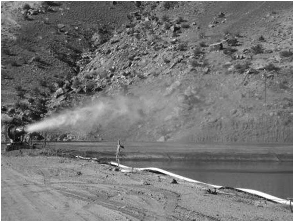
FIGURE 16.40 Spray evaporation pond.
