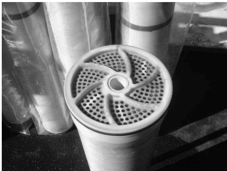
FIGURE 9.4 Coagulant residue on the RO membrane feed due to overdosing.
