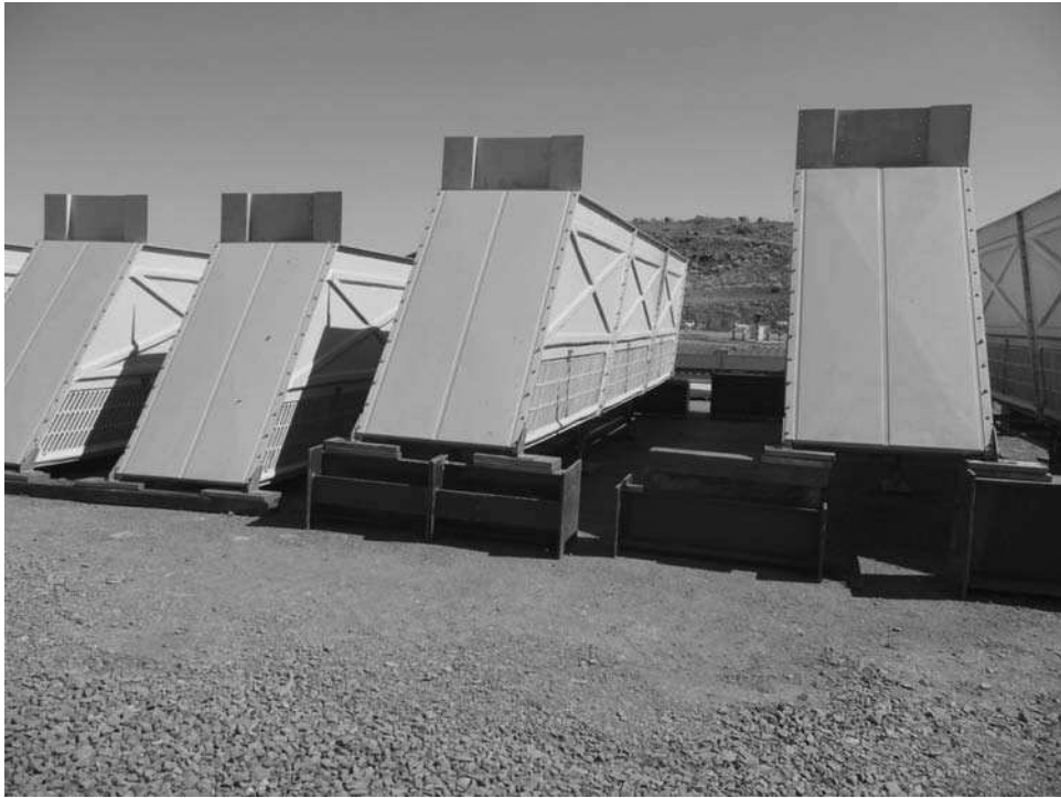
FIGURE 10.3 Lamella modules—Cape Preston desalination plant, Australia.
