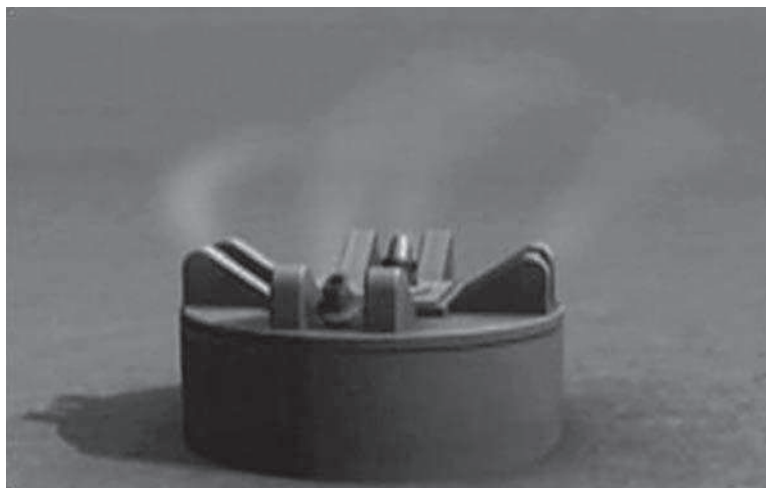
FIGURE 16.6 Sydney water SWRO diffuser structure.
