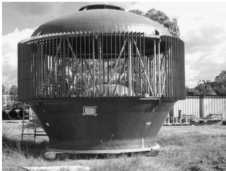
FIGURE 5.1 Intake bar screen. (Source: GHD.)
