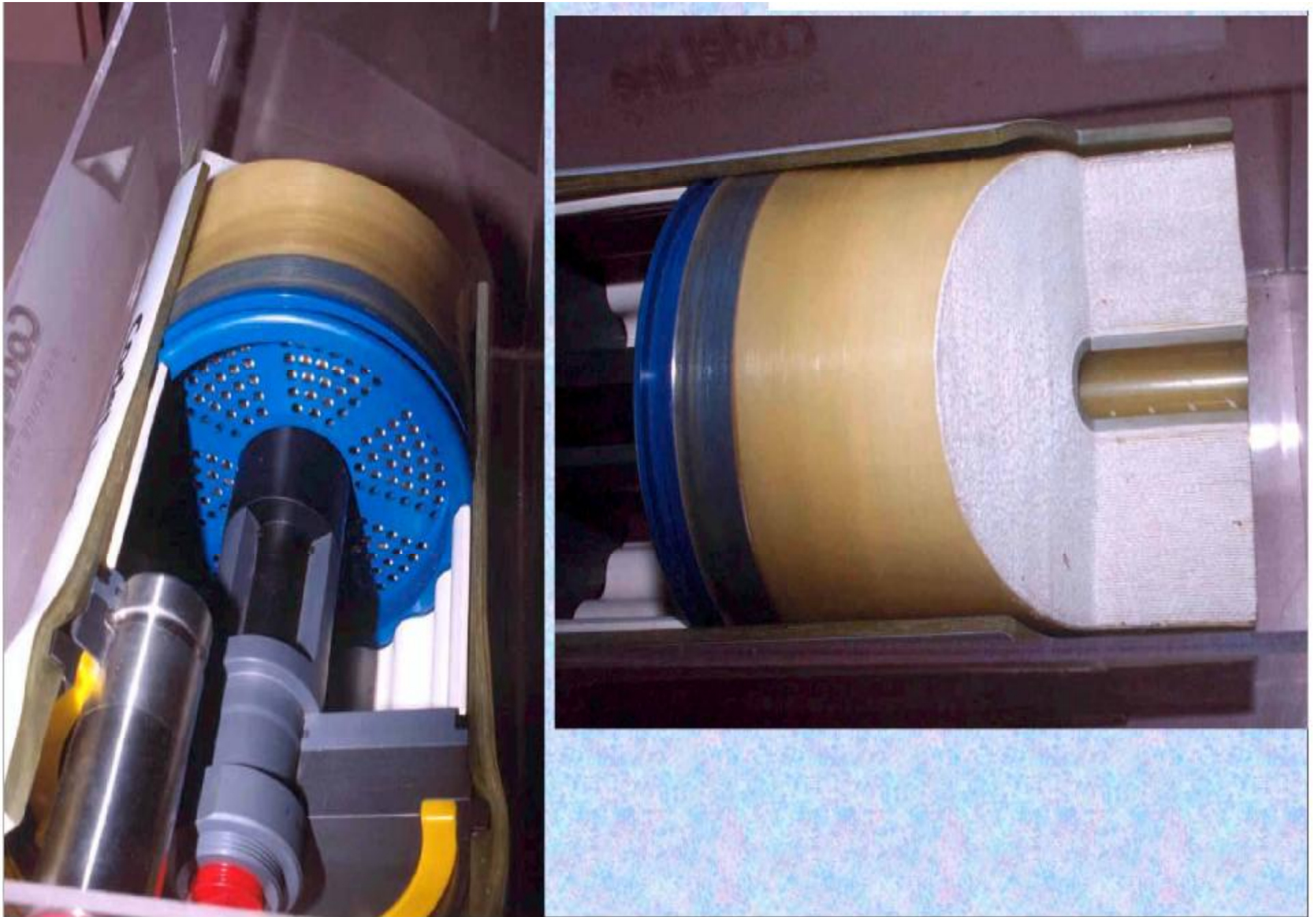
Fig. 4.13 Cut-way photo in a Spiral wound membrane module
