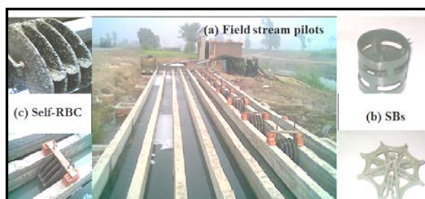
Figure 3: a) The field experimental stream pilots installed at Bilbeas drain; b) Plastic media (Pall rings and Star shape), c) Self-RBC
