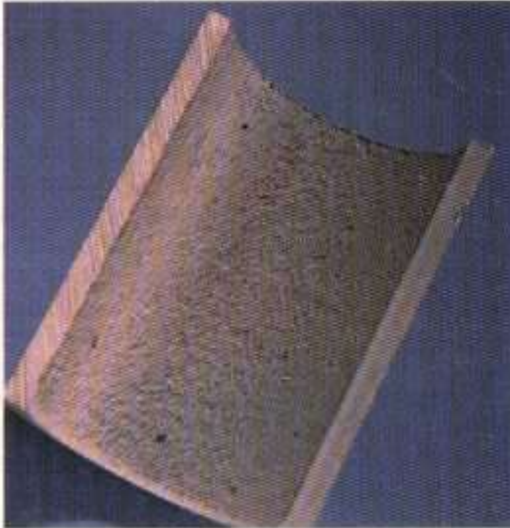
Boiler tube shows effect of acid attack.
