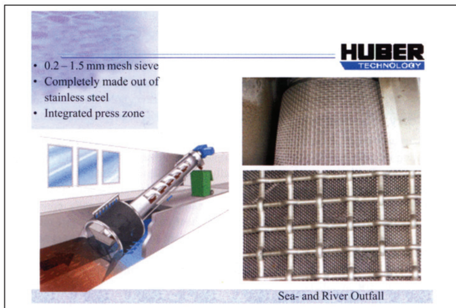
Figure 2: Preliminary Treatment by Rotating Fine Screens
