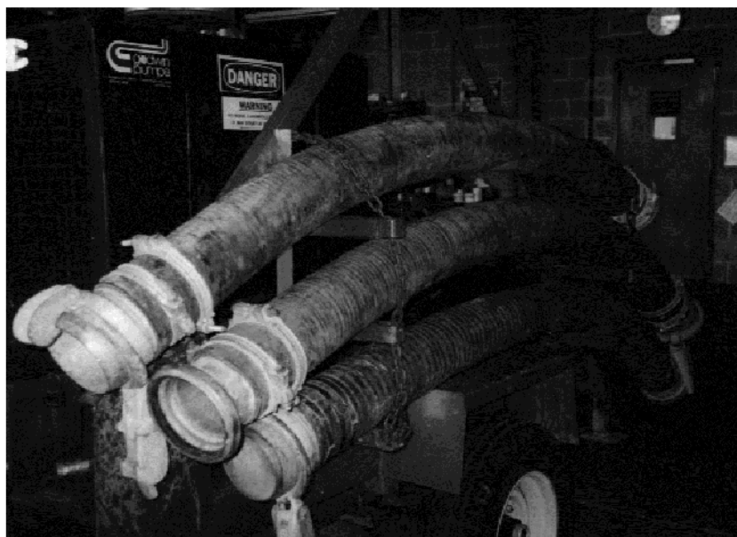
Figure 5.13 Flexible hose with quick-connect couplings.
