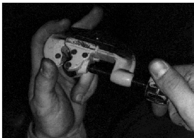
Figure 4.6 Cutting tool used to cut copper tubing.
