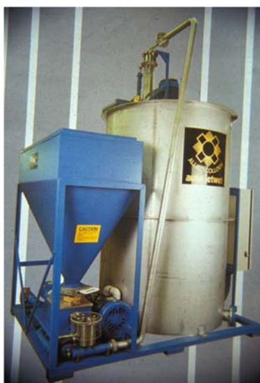
Figure 2 Compact equipment for polyelectrolyte preparation in sludge conditioning.
