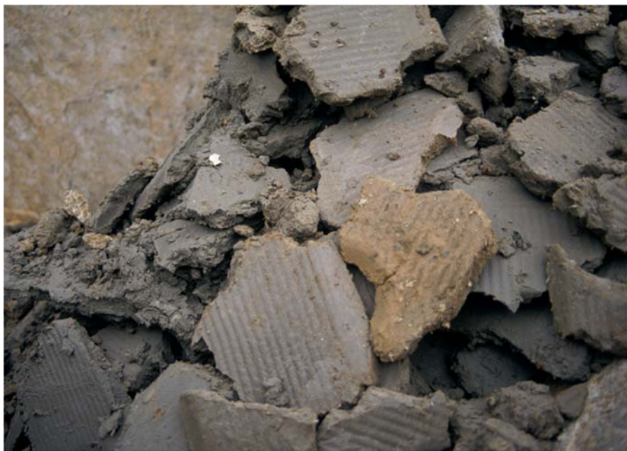
Figure 26. Final appearance of dewatered sludge cake in a press filter.
