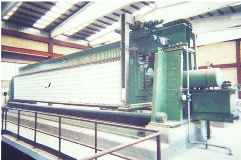
Figure 21. General view of a press filter.
