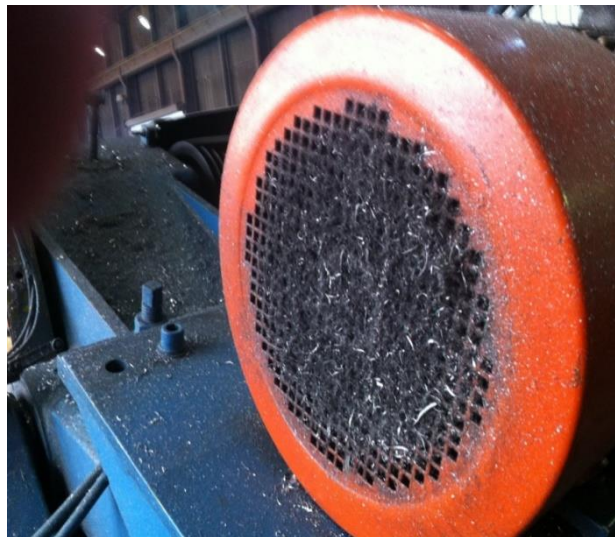
Figure 73 Partially blocked fan on an induction motor in a metal processing plant. (Atkins)
