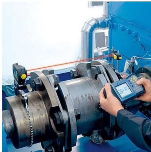
Figure 71 Modern laser alignment equipment (directindustry.com)
