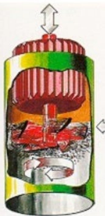
Vertical shot-blasting for large pipes
