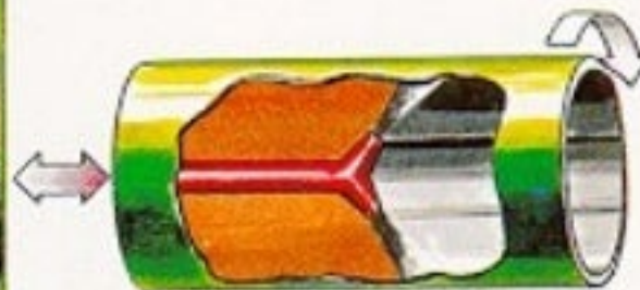
Horizontal shot-blasting for small pipes
