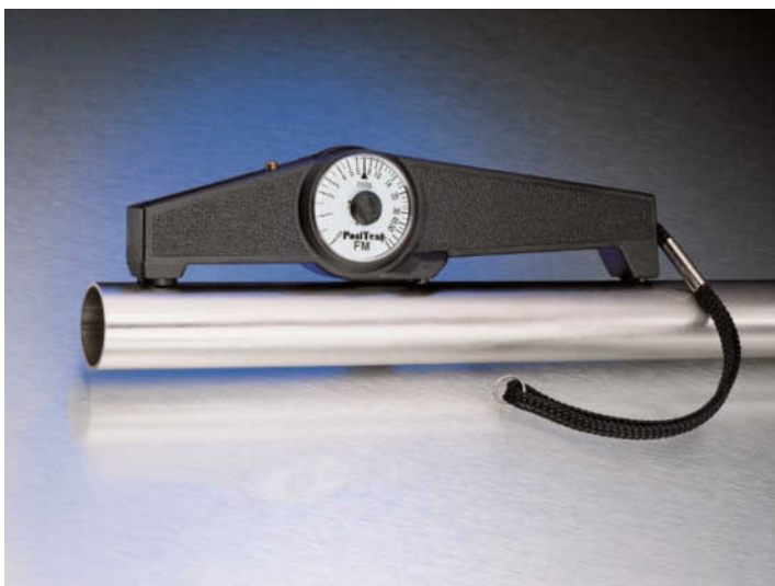
Figure 8-6. Dial-type magnetic pull-off DFT gauge.
