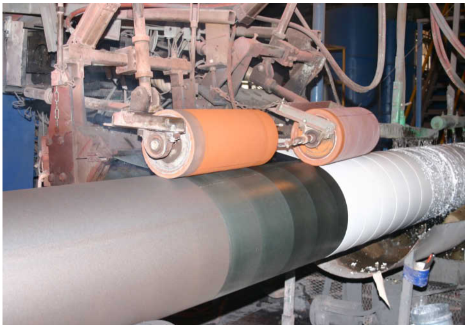
Figure 8-2. Side extrusion for a three-layer coating system.
