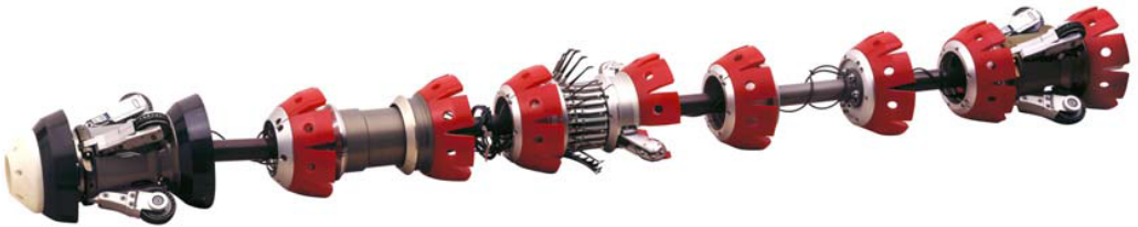
Figure 9-4. In-line current survey tool.
