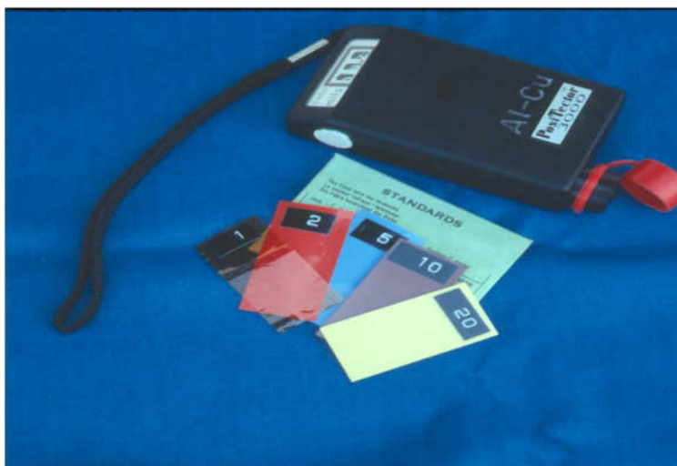
Figure 8-9. Constant-pressure probe gauge calibrated with plastic shims.
