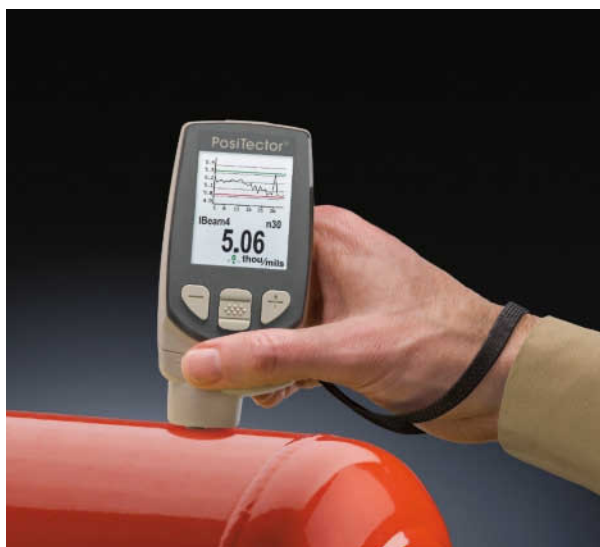
Figure 8-7. Magnetic constant-pressure DFT gauge.
