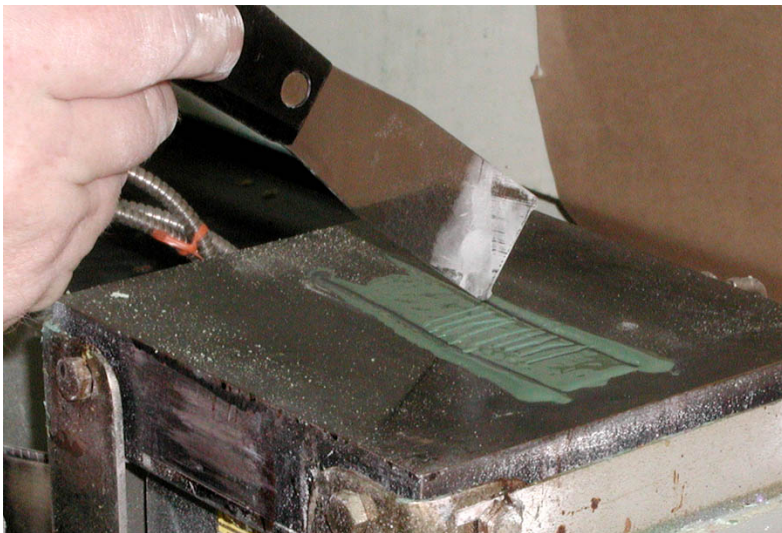
Figure 6-5. FBE powder gel test.
